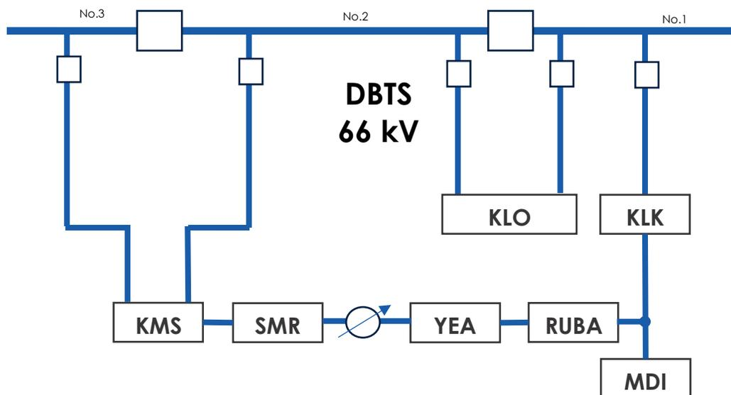
Figure 14: Possible sub-transmission network schematic diagram (Option 6 - SMTS)
