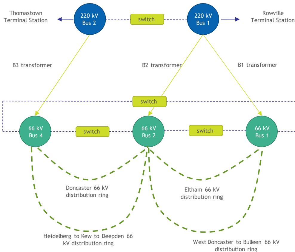
Figure 4 - Representative diagram for TSTS
