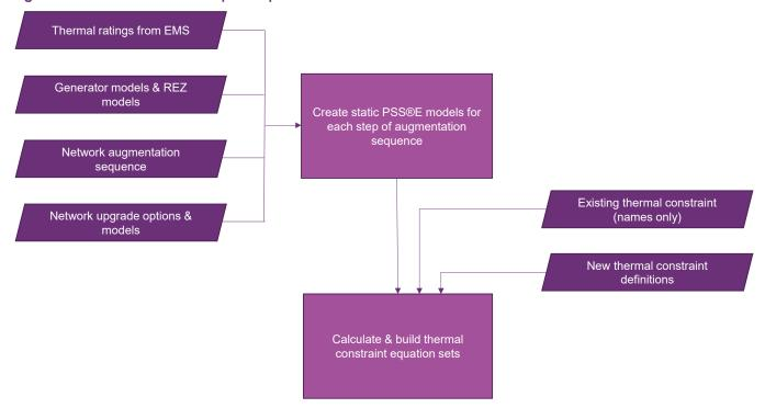
Figure 18 Thermal constraint equation process
