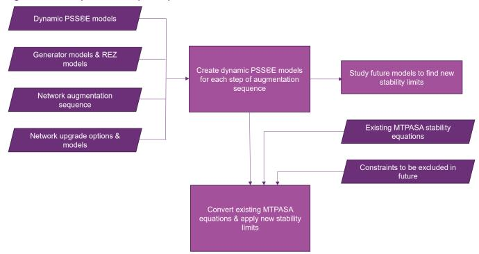
Figure 19 Stability constraint equation process
