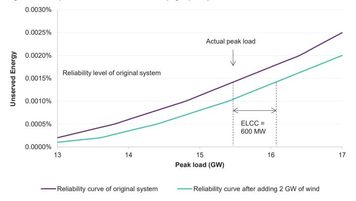
Figure 12 Example calculation of effective load carrying capability
