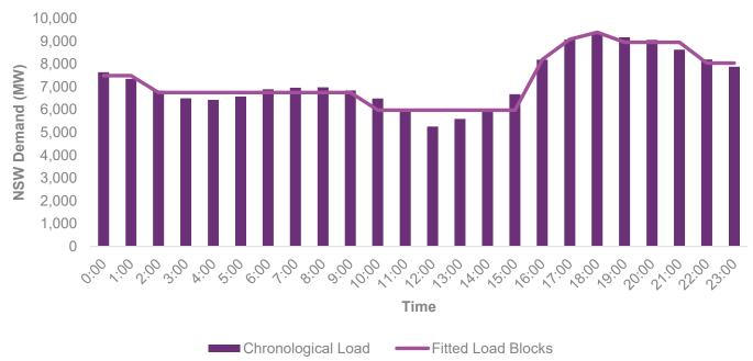
Figure 11 Example representation of fitted load blocks
