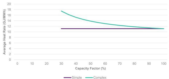
Figure 17 Example of heat rates – simple versus complex
