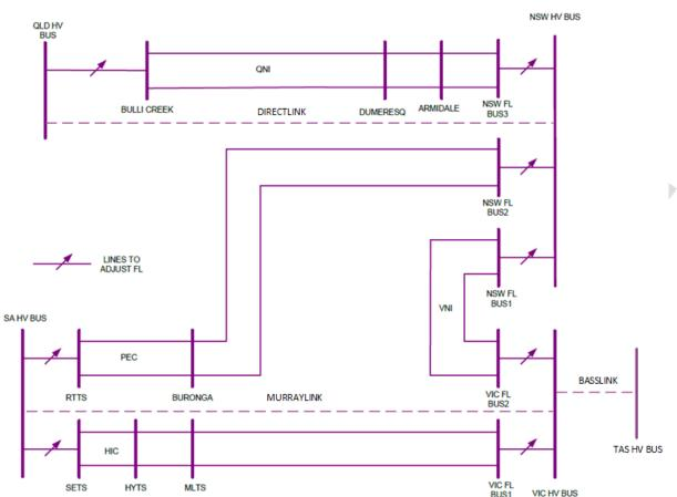
Figure 8 Simplified single line diagram of the updated simplified NEM model with PEC Stage 2 integrated
