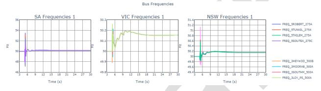
System instability in this case was avoided by the function of the SPS. The design of this scheme is not final, but in the 2022 PSFRR full NEM future case benchmarking studies, the scheme was implemented as follows for South Australia import conditions:
