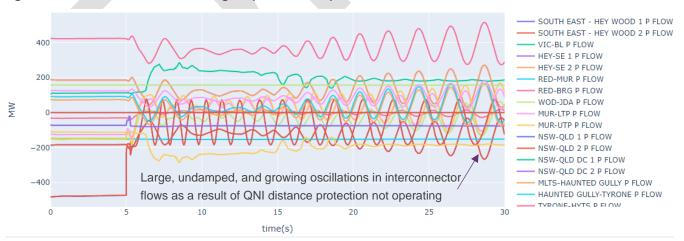
Case 15 was rerun tripping the 132 kV lines between Kempsey and Taree, and Moree and Inverell. The simulation results are shown in the figures below. Queensland successfully separated from the rest of the NEM and Queensland frequency did not fall below 49 Hz or exceed 51 Hz. AUFLS operates in Tasmania, resulting in load shedding.
