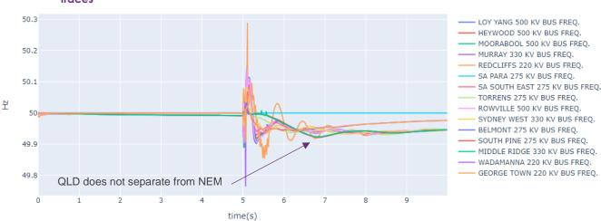
Figure 38 Case 14, Wagga contingency, not inter-tripping Sunraysia SF and Limondale 1 SF: system frequency traces
