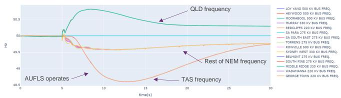
Figure 67 Case 15, Tamworth contingency, 132 kV lines tripped: system frequency traces
