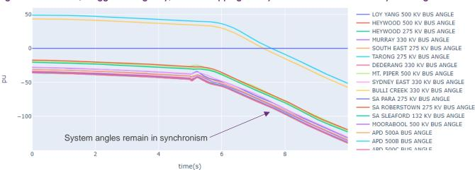
Figure 35 Case 14, Wagga contingency, not inter-tripping Sunraysia SF and Limondale 1 SF: system angles
