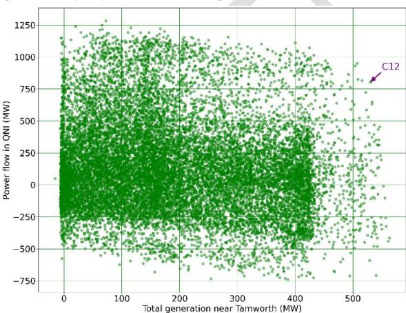
Figure 4 Scatter plot of power flow on QNI and total generation near Tamworth for FY 2021-22
