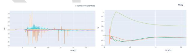
Figure 9 Frequency performance – unstable simplified model (left) vs stable full model (right)
