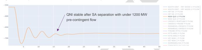
In the full OPDMS model, QNI appeared to enter an unstable condition almost immediately after exceeding its export limit of 1,200 MW, at 1,400 MW. In the simplified model, however, QNI reached a peak flow of 1,460 MW with no instability and reached a settled point of 1,350 MW. QNI appeared to remain stable for this condition regardless of tuning.
