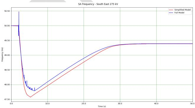
The frequency decline triggered in South Australia in the simplified model as a result of the separation cannot be attributed to 7 MW of additional DPV tripping due to voltage protection. It appears as though frequency movements in South Australia are generally exaggerated in the simplified model compared to the OPDMS full NEM model. As synchronous regional inertia is identical in both models, a number of factors could be causing this, including:
