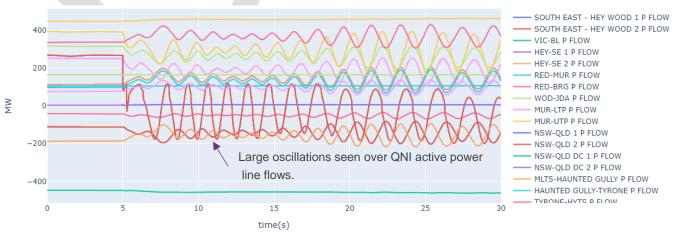
Case 8 was rerun tripping the 132 kV lines between Kempsey and Taree, and Moree and Inverell. The simulation results are shown in the figures below. Queensland successfully separated from the rest of the NEM and Queensland frequency did not fall below 49 Hz or exceed 51 Hz.
