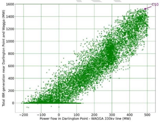
Figure 3 Scatter plot of total IBR generation in New South Wales and power flow on Darlington Point – Wagga 330 kV line for FY 2021-22
