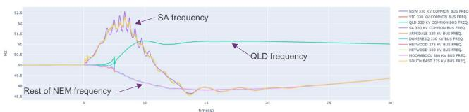
Figure 78 Case 9, South Australia separation at MLTS with APD load tripping: system frequency traces
