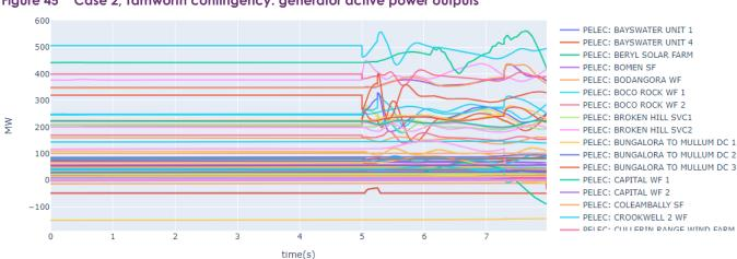
Figure 45 Case 2, Tamworth contingency: generator active power outputs
