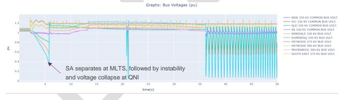
Figure 18 Full OPDMS PSS®E model, SA separation at MLTS, Export Case 1
