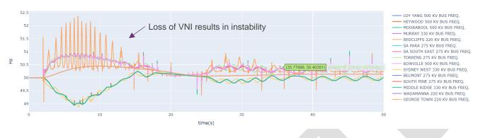
Figure 23 Simplified PSS®E model, VNI separation, Export Case 1
