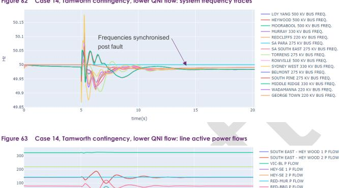
Figure 62 Case 14, Tamworth contingency, lower QNI flow: system frequency traces
