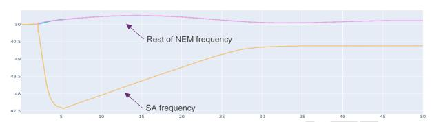
Figure 15 Simplified PSS®E model, SA frequency, SA separation at HYTS, Import Case 1
