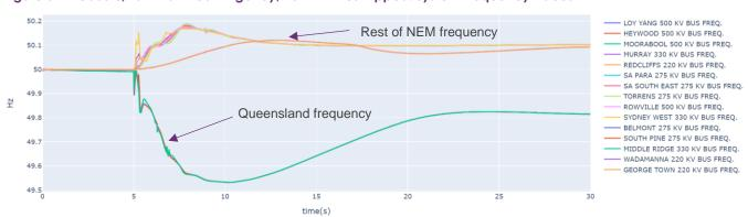
Figure 51 Case 8, Tamworth contingency, 132 kV lines tripped: system frequency traces
