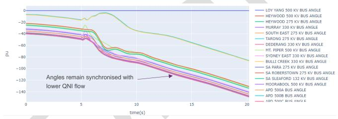
Figure 60 Case 14, Tamworth contingency, lower QNI flow: system angles
