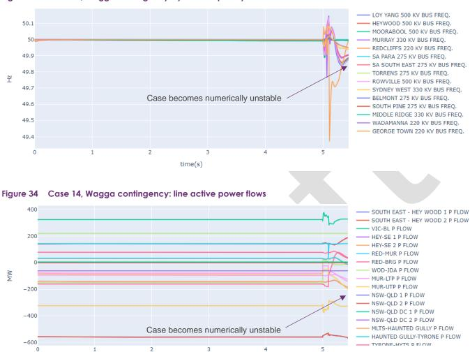
Figure 33 Case 14, Wagga contingency: system frequency traces
