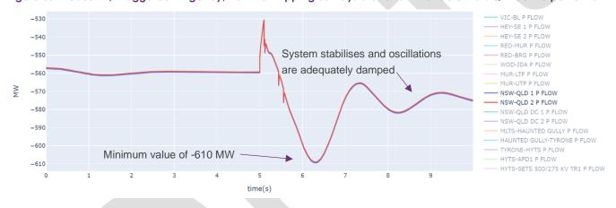
Figure 37 Case 14, Wagga contingency, not inter-tripping Sunraysia SF and Limondale 1 SF: generator active power outputs
