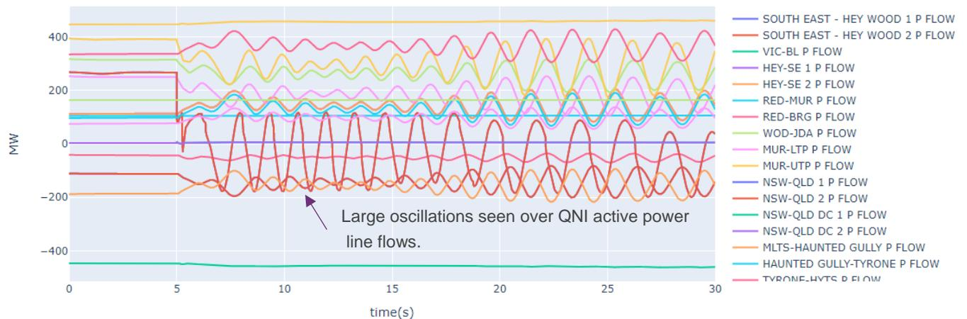
Case 8 was rerun tripping the 132 kV lines between Kempsey and Taree, and Moree and Inverell. The simulation results are shown in the figures below. Queensland successfully separated from the rest of the NEM and Queensland frequency did not fall below 49 Hz or exceed 51 Hz.
