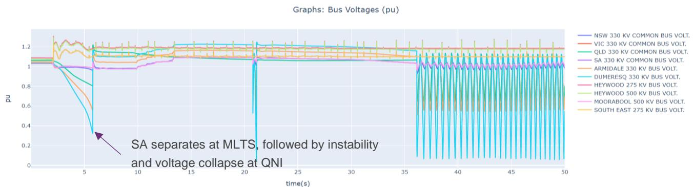
Figure 18 Full OPDMS PSS®E model, SA separation at MLTS, Export Case 1
