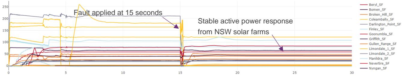
Figure 41 Case 4, Wagga contingency, PSCAD™ results: NSW solar farm reactive power outputs
