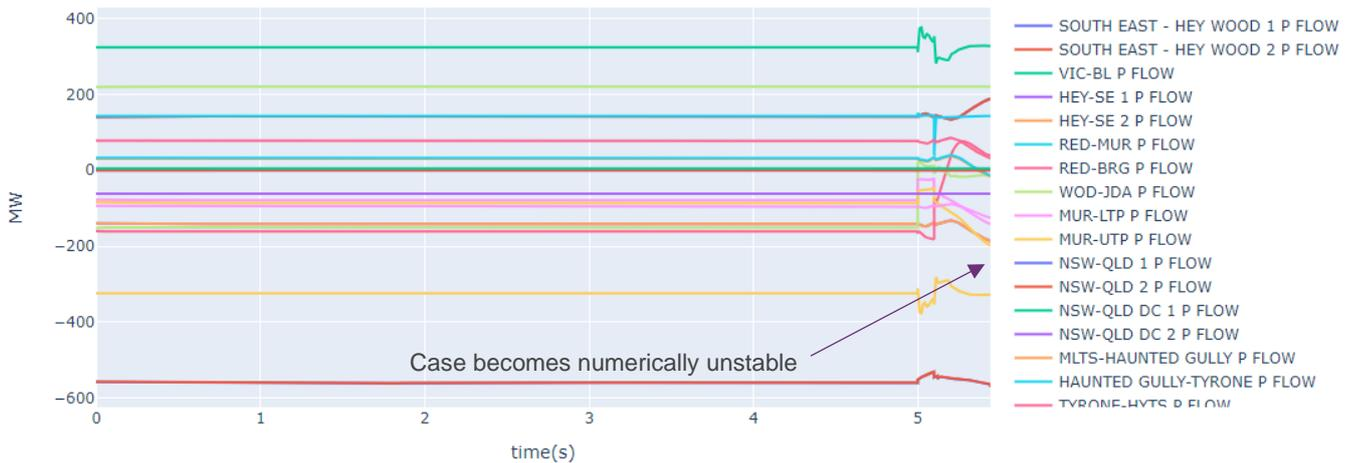
Case 14 was rerun with approximately 300 MW less generation being inter-tripped by the relevant control schemes, and the case completes without Queensland separating from the rest of the NEM – see plot of system angles below. The simulation results are shown in the figures below.
