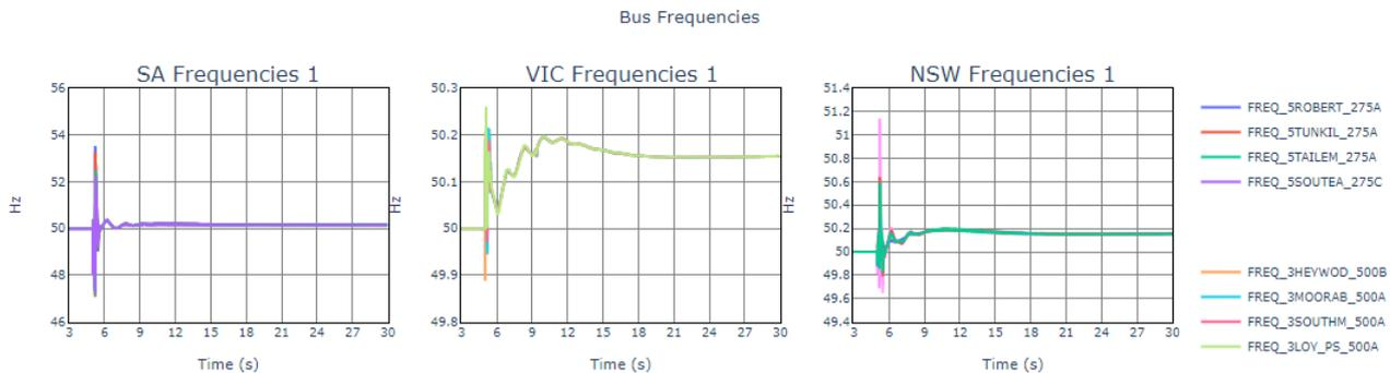
System instability in this case was avoided by the function of the SPS. The design of this scheme is not final, but in the 2022 PSFRR full NEM future case benchmarking studies, the scheme was implemented as follows for South Australia import conditions:
