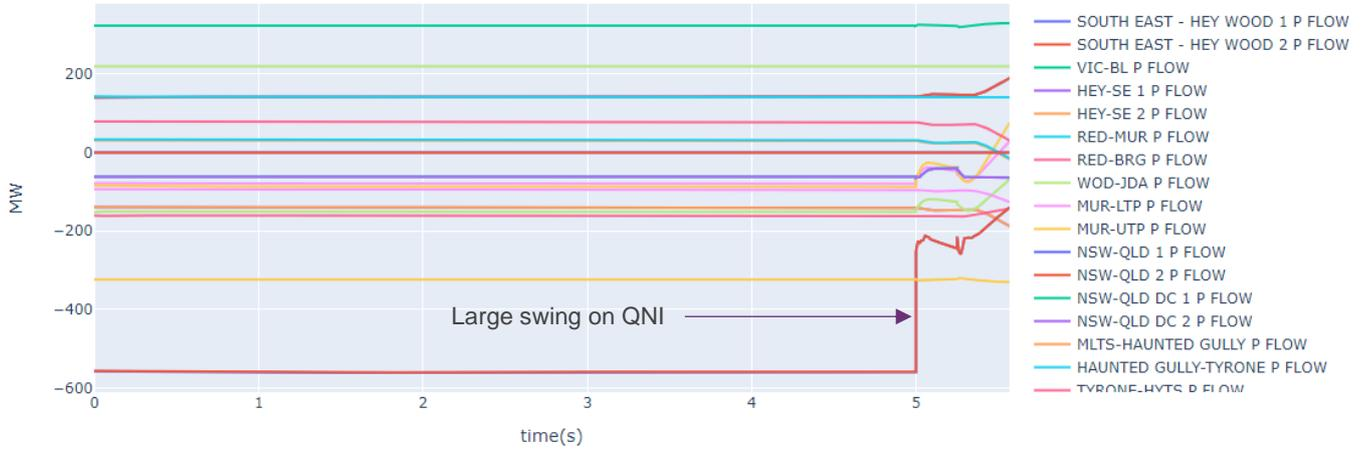
Case 14 was rerun with reduced QNI flow (transfer was approximately 100 MW), the case completed and QNI remained stable following fault clearance. The simulation results are shown in the figures below.
