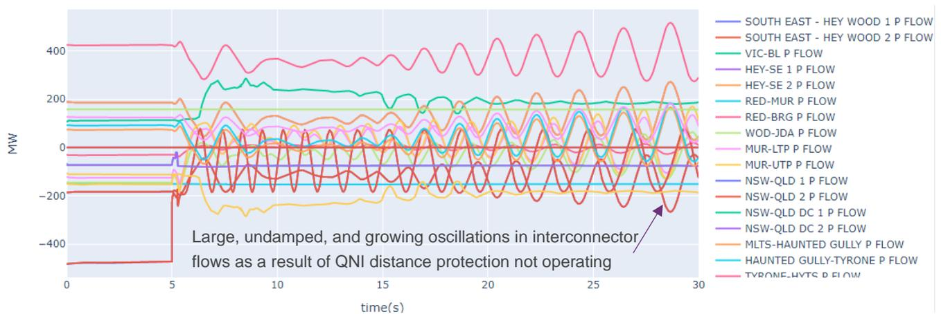
Case 15 was rerun tripping the 132 kV lines between Kempsey and Taree, and Moree and Inverell. The simulation results are shown in the figures below. Queensland successfully separated from the rest of the NEM and Queensland frequency did not fall below 49 Hz or exceed 51 Hz. AUFLS operates in Tasmania, resulting in load shedding.
