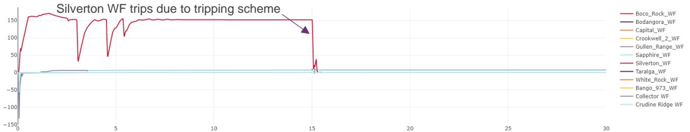
Figure 43 Case 4, Wagga contingency, PSCAD™ results: NSW wind farm reactive power outputs
