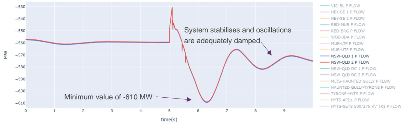
Figure 37 Case 14, Wagga contingency, not inter-tripping Sunraysia SF and Limondale 1 SF: generator active power outputs
