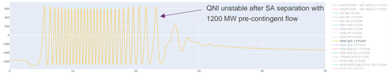
**Figure 12** Simplified PSS®E model, QNI power flow, SA separation at HYTS, Export Case 11
