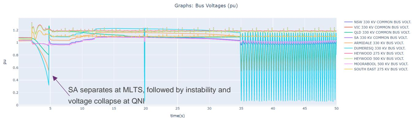
**Figure 20 Full OPDMS PSS@E model, SA separation at MLTS, Export Case 3**
