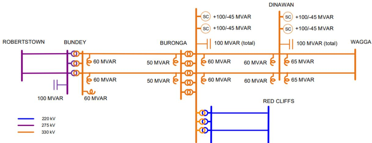
To enable studies with future operating conditions for FY 2027-28, PEC Stage 2 was integrated into the future simplified NEM model. The PEC Stage 2 model was integrated with the simplified model with connections between Robertstown and South Australia fault level buses established, and between Wagga Wagga and New South Wales fault level buses established, thereby allowing for power transfers between New South Wales and South Australia via the interconnector.
