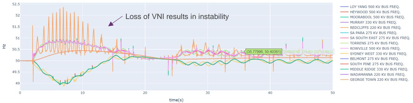
Figure 23 Simplified PSS@E model, VNI separation, Export Case 1
