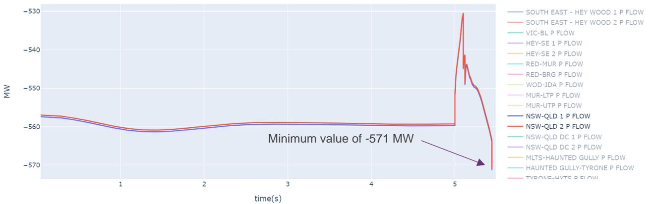
Figure 32 Case 14, Wagga contingency: generator active power outputs
