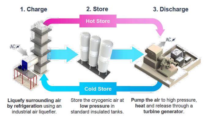
Additional hot and cold thermal recycling increases efficiency
