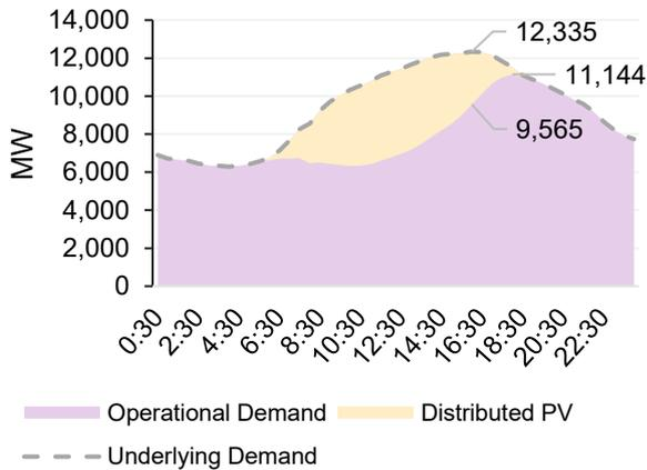
**Figure 11 South Australian maximum demand period shifted later into the evening due to distributed PV generation**
