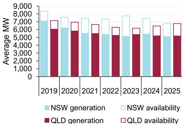
**Figure 32 Return of Callide C reduced Queensland black coal-fired capacity on full outage**
