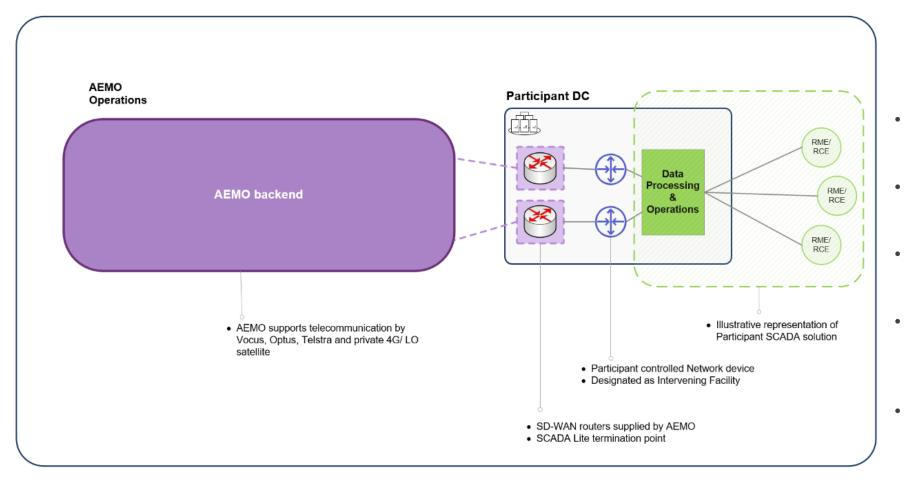
Dual Cisco SD-WAN routers installed in secure location inside data centre
