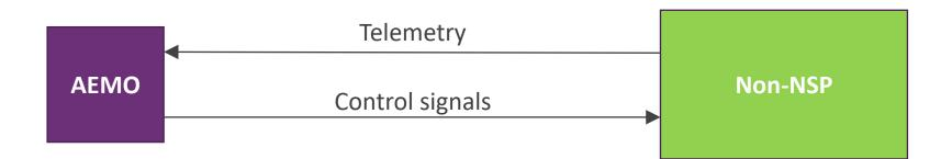
SCADA Lite will enable NEM non-NSP Participants to establish a bi-directional connection to exchange operational information (telemetry and control) with AEMO.
