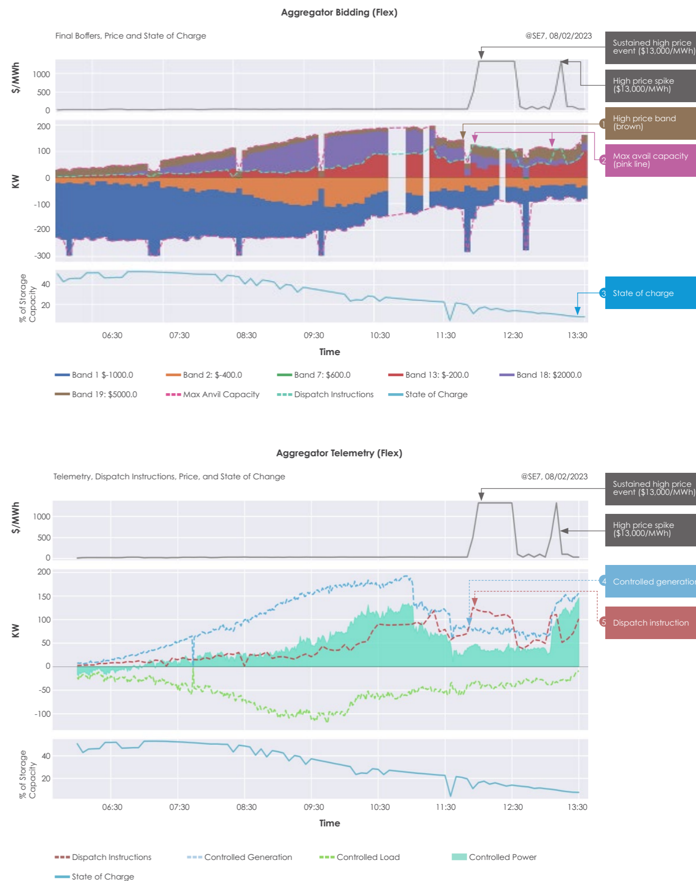
Figure 62 | Testing of aggregator response to a sustained high price during midday followed by a spike
