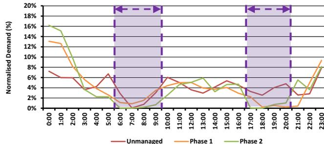
Source: AGL, Energeia Analysis. Note: Unmanaged: 10 chargers, Phase 1: 11 chargers, Phase 2: 8 22 kW chargers. Evening period start and end time varies up to half an hour by state. Purple indicates smart charging period. Morning period occurs in Phase 2 only
