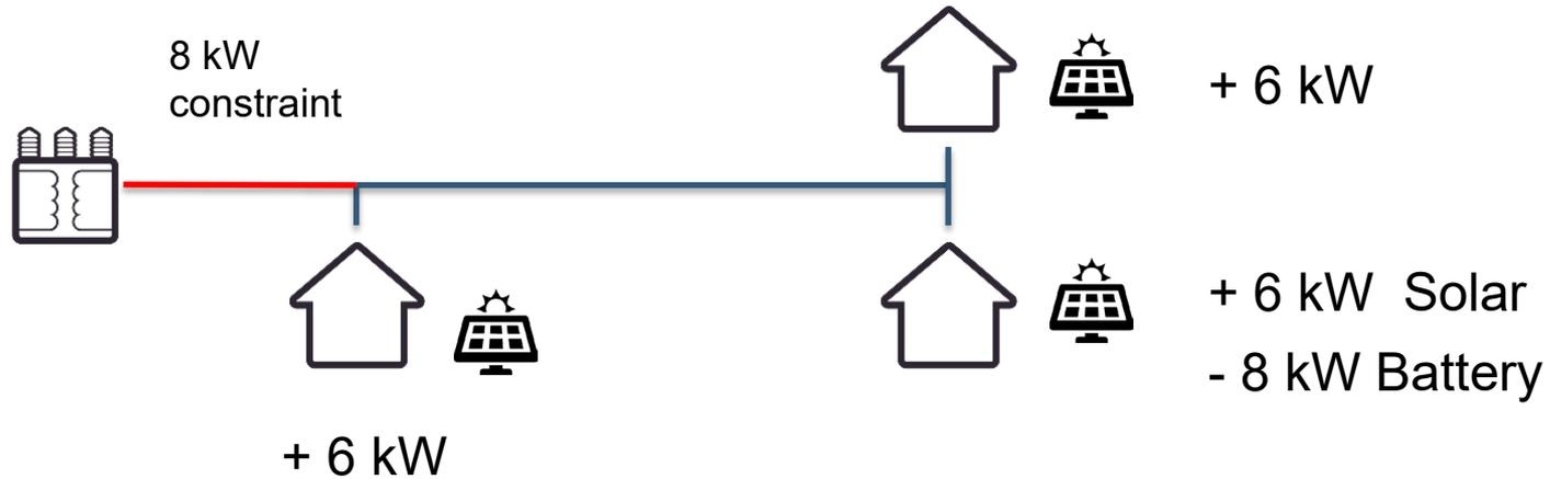
DOEs allocated at transformer level would give an export envelope of  $8/3$  kW (2.67kW).
