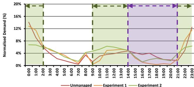
Source: Origin, Energeia Analysis. Note: Unmanaged: 13 vehicles, Exp 1: 13 vehicles, Exp 2: 13 vehicles. Green indicates incentive to charge, purple indicates controlled charging (Experiment 2 only)
