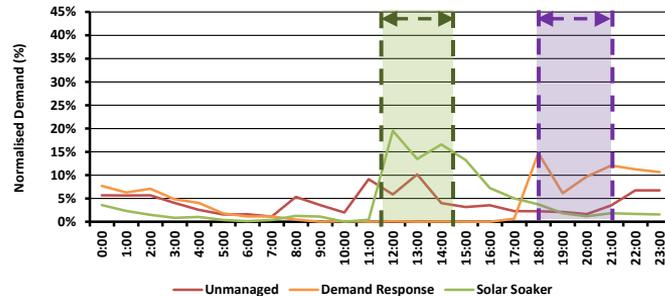
Source: EV Grid. Note: Green indicates incentive to charge, Purple indicates controlled charging. Unmanaged: 26 vehicles, Demand Response: 17 vehicles, Solar Soaker: 19 vehicles.
