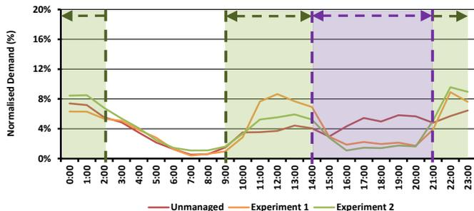
Source: Origin, Energeia Analysis. Note: Unmanaged: 26 vehicles, Exp 1: 26 vehicles, Exp 2: 26 vehicles. Green indicates charging incentive, purple indicates controlled charging (Experiment 2 only)
