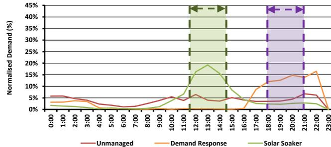
Source: EV Grid, Energeia. Note: Green indicates incentive to charge, Purple indicates controlled charging. Unmanaged: 117 chargers, Demand Response: 80 chargers, Solar Soaker: 91 chargers.
