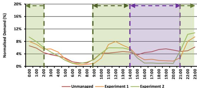
Source: Origin, Energeia Analysis. Note: Unmanaged: 54 vehicles, Exp 1: 55 vehicles, Exp 2: 57 vehicles. Green indicates charging incentive, purple indicates controlled charging (Experiment 2 only)
