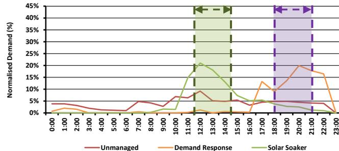
Source : EV Grid, Energeia , Note: Green indicates incentive to charge, Purple indicates controlled charging. Unmanaged: 41 chargers, Demand Response: 22 chargers, Solar Soaker: 32 chargers.
