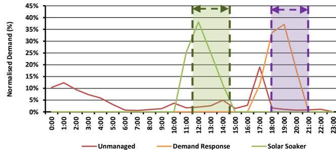
Source: EV Grid. Note: Green indicates incentive to charge, Purple indicates controlled charging. Unmanaged: 4 chargers, Demand Response: 1 charger, Solar Soaker: 3 chargers.
