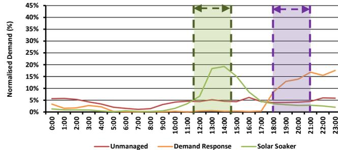
Source: EV Grid. Note: Green indicates incentive to charge, Purple indicates controlled charging. Unmanaged: 137 vehicles, Demand Response: 87 vehicles, Solar Soaker: 107 vehicles.
