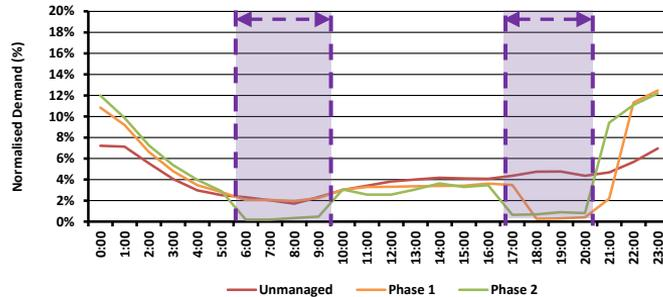
Source: AGL, Energeia Analysis. Note: Unmanaged: 106 chargers, Phase 1: 110 chargers, Phase 2: 89 22 kW chargers. Evening period start and end time varies up to half an hour by state. Purple indicates smart charging period. Morning period occurs in Phase 2 only
