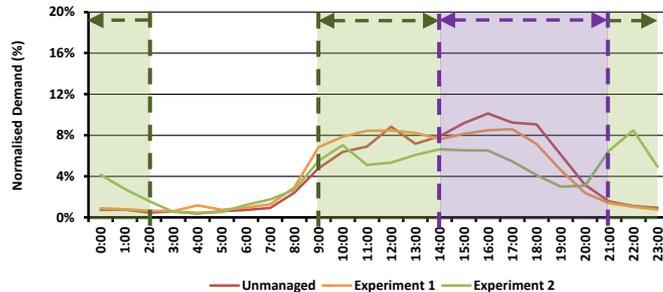
Source: Origin, Energeia Analysis. Note: Unmanaged: 25 vehicles, Exp 1: 26 vehicles, Exp 2: 53 vehicles. Green indicates charging incentive, purple indicates controlled charging (Experiment 2 only)
