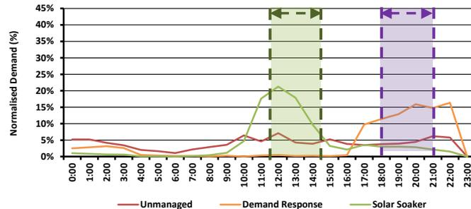
Source: EV Grid. Note: Green indicates incentive to charge, Purple indicates controlled charging. Unmanaged: 160 chargers, Demand Response: 104 chargers, Solar Soaker: 88 chargers.
