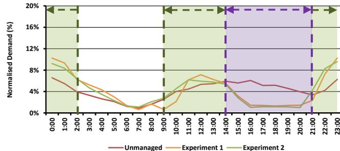
Source: Origin, Energeia Analysis. Note: Unmanaged: 59 vehicles, Exp 1: 60 vehicles, Exp 2: 62 vehicles. Green indicates incentive to charge, purple indicates controlled charging (Experiment 2 only)
