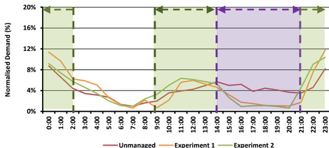
Source: Origin, Energeia Analysis. Note: Unmanaged: 39 vehicles, Exp 1: 40 vehicles, Exp 2: 42 vehicles. Green indicates charging incentive, purple indicates controlled charging (Experiment 2 only)
