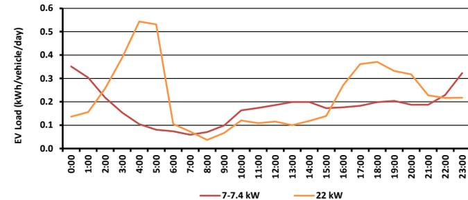
Source: AGL, Origin. Note: 5 22kW chargers, 62 7-7.4 kW chargers. Early morning spike caused by single charger.
