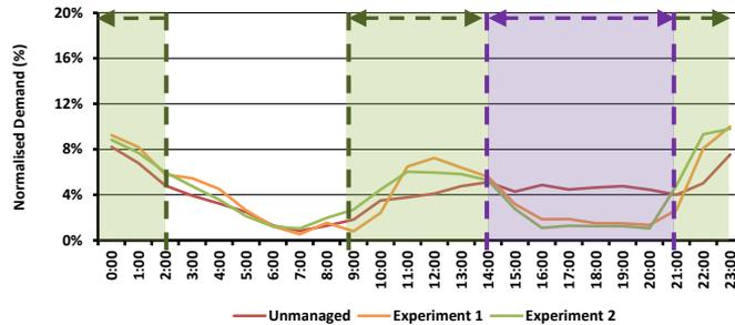
Source: Origin, Energeia Analysis. Note: Unmanaged: 67 vehicles, Exp 1: 68 vehicles, Exp 2: 70 vehicles. Green indicates charging incentive, purple indicates controlled charging (Experiment 2 only)
