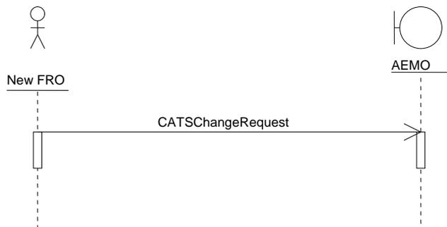
FIGURE 4-2. INITIATING TRANSFER REQUEST SEQUENCE DIAGRAM
