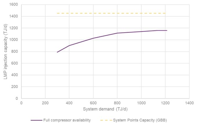
Figure 34 LMP injection capacity to Melbourne (TJ/d)
