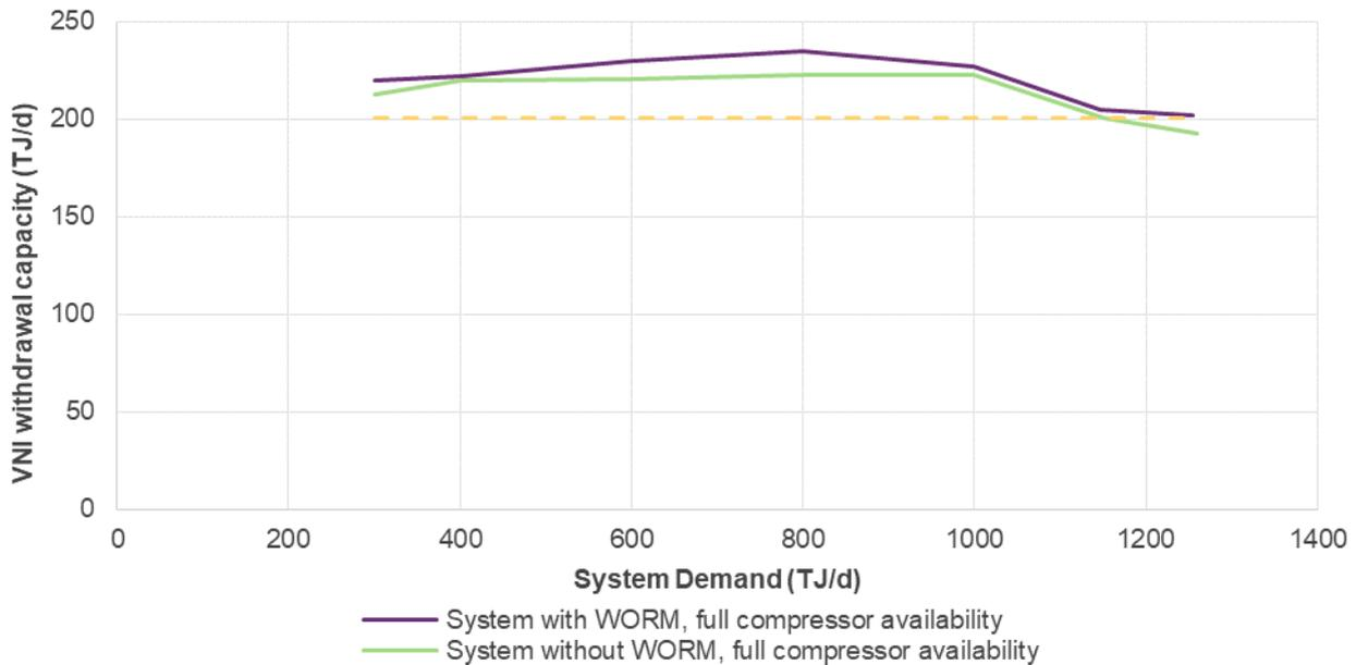
The increase in capacity for system demands between 300 TJ/d and 400 TJ/d is relatively small, as two Wollert compressors are sufficient to maintain the Wollert outlet pressure close to the maximum discharge pressure. The
