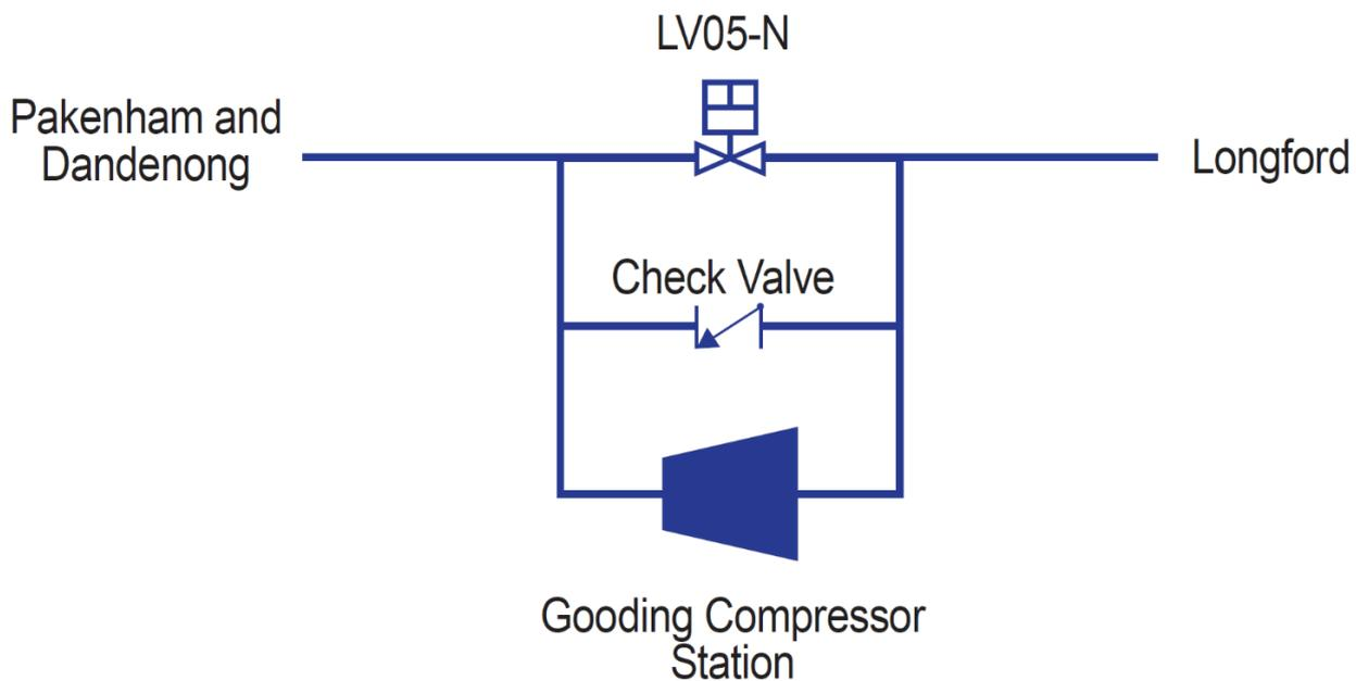
In the event of insufficient injections at Longford CPP, LV05N will need to be opened to allow easterly flow at Gooding. The valve will need to be closed again to enable Gooding compression. To remove the requirement for APA site attendance every time easterly flow is required, modification to this valve or elsewhere in the station should be undertaken to enable remote operation by AEMO and APA.
