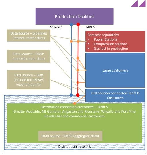
Figure 1 Logical schematic of South Australian gas network
