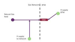
Hydrogen supply either through existing gas network or by new behind-themeter facilities will offset natural gas use. This applies for cases with constant gas demand, and for cases with expected growth in gas demand.
