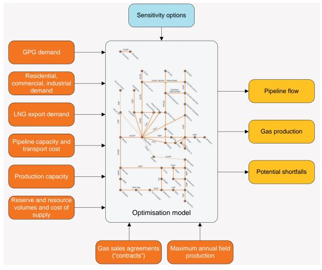
The eastern and south-eastern gas network is represented by a series of connected nodes. At each node, gas may be injected into or withdrawn from the network, or flow may be redirected.
