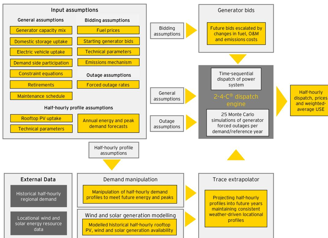
Figure 2: Data flow diagram for the market simulations
