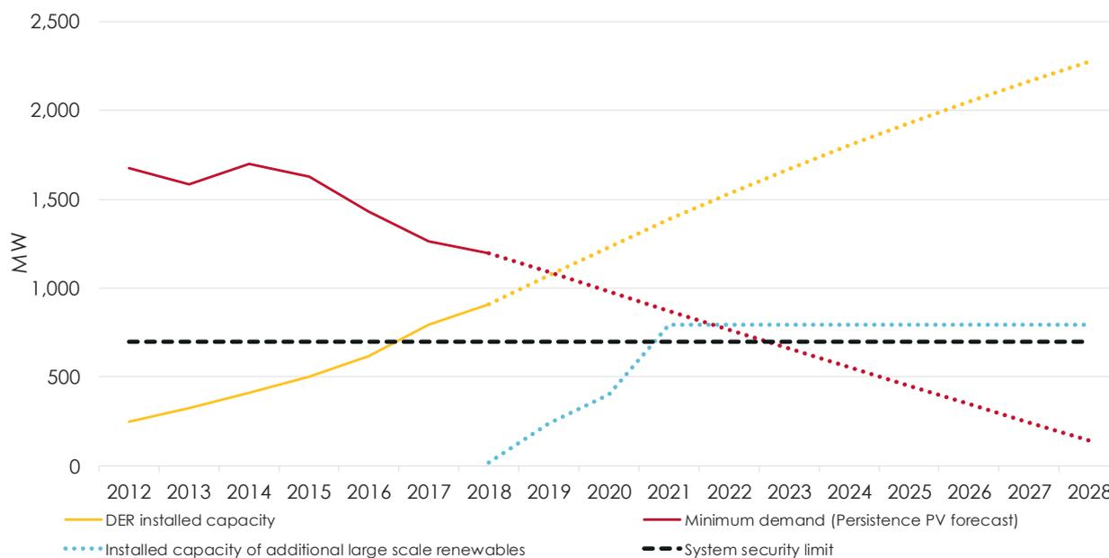
Figure 3 shows the minimum operational demand and DER capacity. In 2022 the level of minimum operational demand will potentially breach the system security threshold of 700 MW. In this year, DER will potentially supply 62% of underlying demand in the Trading Interval with the maximum DER penetration.
