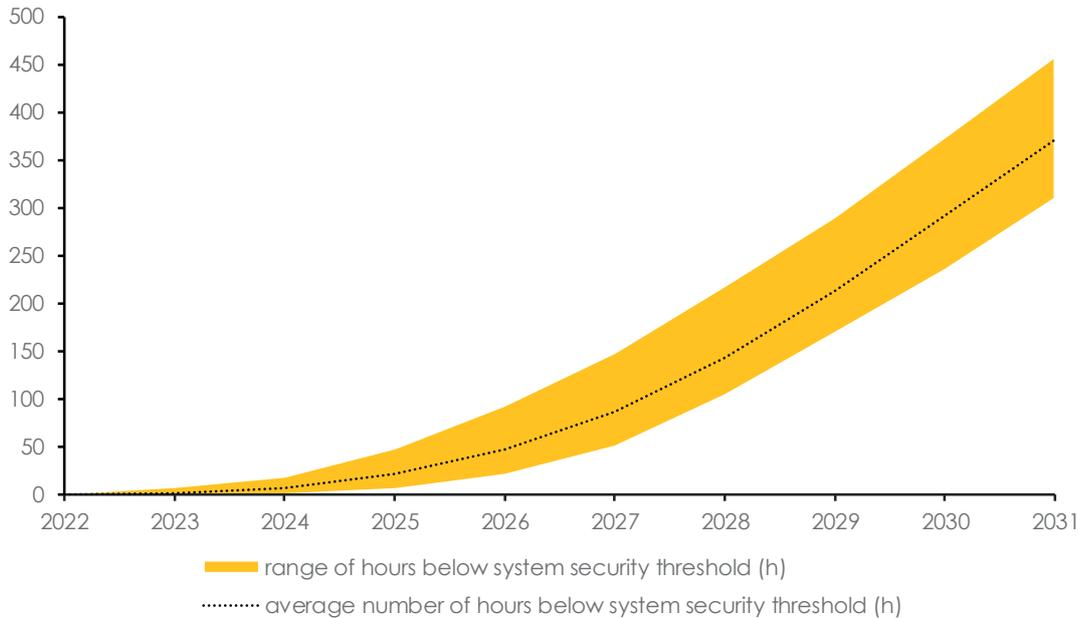
In as early as 2022, the system security threshold could be breached in up to 10 hours of the year; by the end of 2024, the system is insecure in up to 50 hours; by the end of 2030, this number increases to 460 hours (more than 19 days) of the year. This reflects the escalation of challenges for the secure and reliable operation of the power system.
