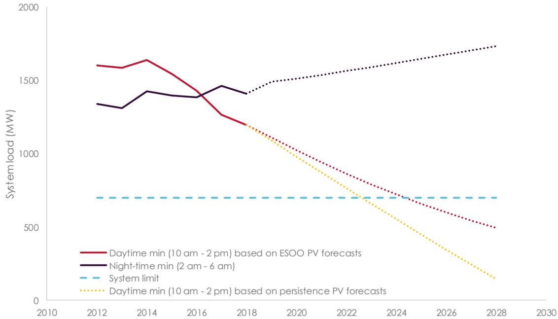
AEMO’s forecasts that considered day-to-day variations in load and rooftop PV generation involved multiple simulations to account for forecast variability. Figure 7 shows the range of hours in a year where SWIS operational demand is projected to be below the 700 MW system security threshold. The dotted line represents the average across the simulated outcomes.
