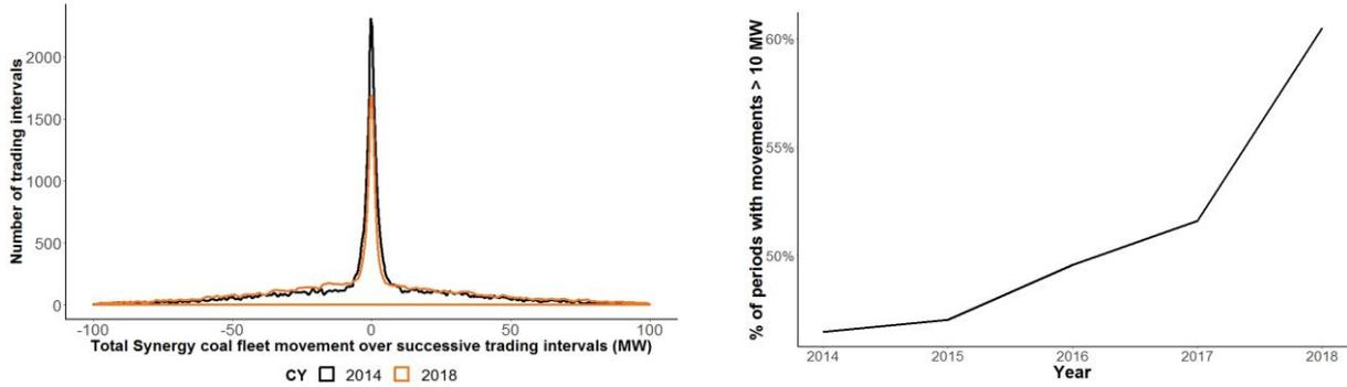
**Figure 15 Synergy coal fleet movements in successive trading intervals, by Facility, 2014 vs 2018**
