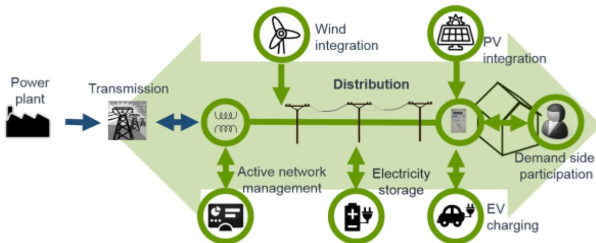
In the evolved electricity system, electricity can flow in a bi-directional manner, that is, flowing to consumers connected to the distribution network, or from the distribution network to the transmission network when generation from DER sources connected to the distribution exceeds customer demand in specific suburbs or substations. This is often referred to as reverse power flow (because it is reverse to the traditional direction of power flow).
