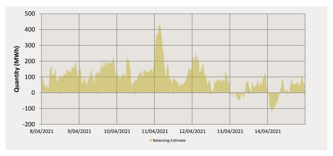
The majority of the balancing activity this week occurred within Balancing Demand. The maximum balancing demand for the week reached 427.3325 MWh on the 11/4/2021. The maximum balancing supply for the week reached -130.142 MWh on the 14/4/2021.
