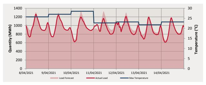
The maximum temperatures for this trading week ranged from  $21.8^{\circ}$ C to  $28.5^{\circ}$ C. The actual load peaked at 1263.96 MWh on the 8/4/2021.
