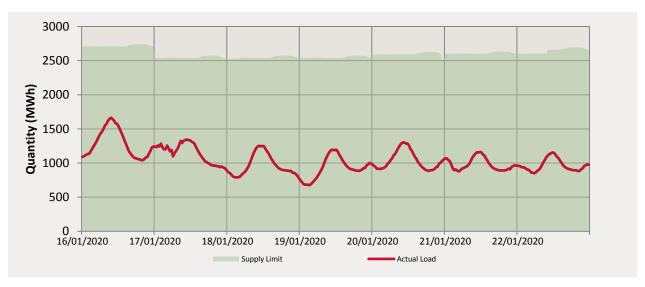
The supply limit ranged from 2490.277 MWh to 2740.94 MWh
