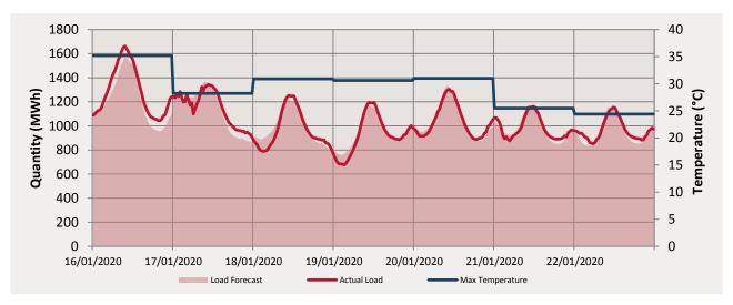
The maximum temperatures for this trading week ranged from  $24.4^{\circ}$ C to  $35.2^{\circ}$ C. The actual load peaked at 1662.919 MWh on the 16/1/2020.
