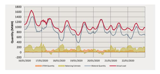
Total balancing supply equalled -1472.505 MWh whereas total balancing demand equalled 43395.945 MWh. The Total STEM Traded quantity was 17200.528 MWh, with the STEM Clearing Quantity ranging between 6.67 MWh and 145.077 MWh.
