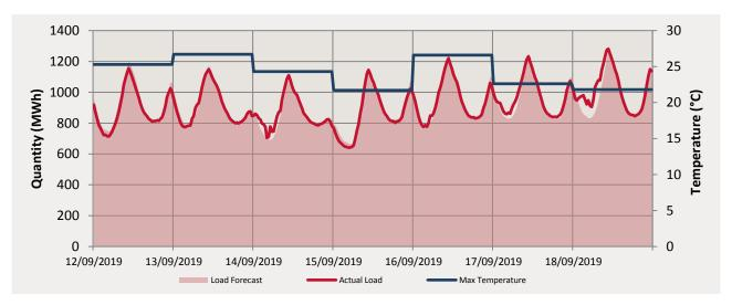
The maximum temperatures for this trading week ranged from  $21.7^{\circ}$ C to  $26.7^{\circ}$ C. The actual load peaked at 1281.481 MWh on the 18/9/2019.
