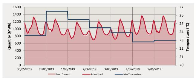
The maximum temperatures for this trading week ranged from 22.8 °C to 26.5 °C. The actual load peaked at 1356.34 MWh on the 4/6/2019.
