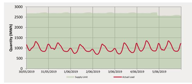
The supply limit ranged from 2569.105 MWh to 2727.717 MWh
