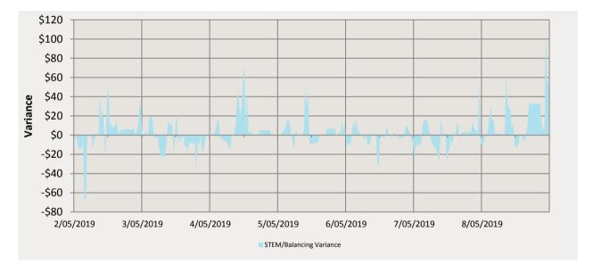
The maximum STEM price was \$80.88/MWh on the 5/5/2019 and the minimum STEM Price recorded was \$-5.48/MWh on the 8/5/2019. The maximum Balancing price was \$151.91/MWh on the 8/5/2019 and the minimum Balancing price recorded was \$-43.57/MWh which occurred on the 2/5/2019.
