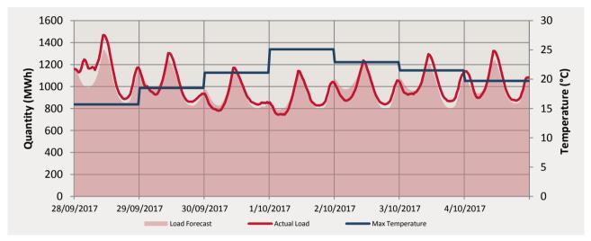
The maximum temperatures for this trading week ranged from 15.7°C to 25.1°C. The actual load peaked at 1467.688 MWh on the 28/9/2017.
