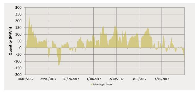
The majority of the balancing activity this week occurred within Balancing Demand. The maximum balancing demand for the week reached 236.321 MWh on the 28/9/2017. The maximum balancing supply for the week reached -132.659 MWh on the 29/9/2012.
