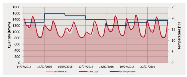
The maximum temperatures for this trading week ranged from 16.8°C to 22°C. The actual load peaked at 1547.362 MWh on the 19/7/2016.
