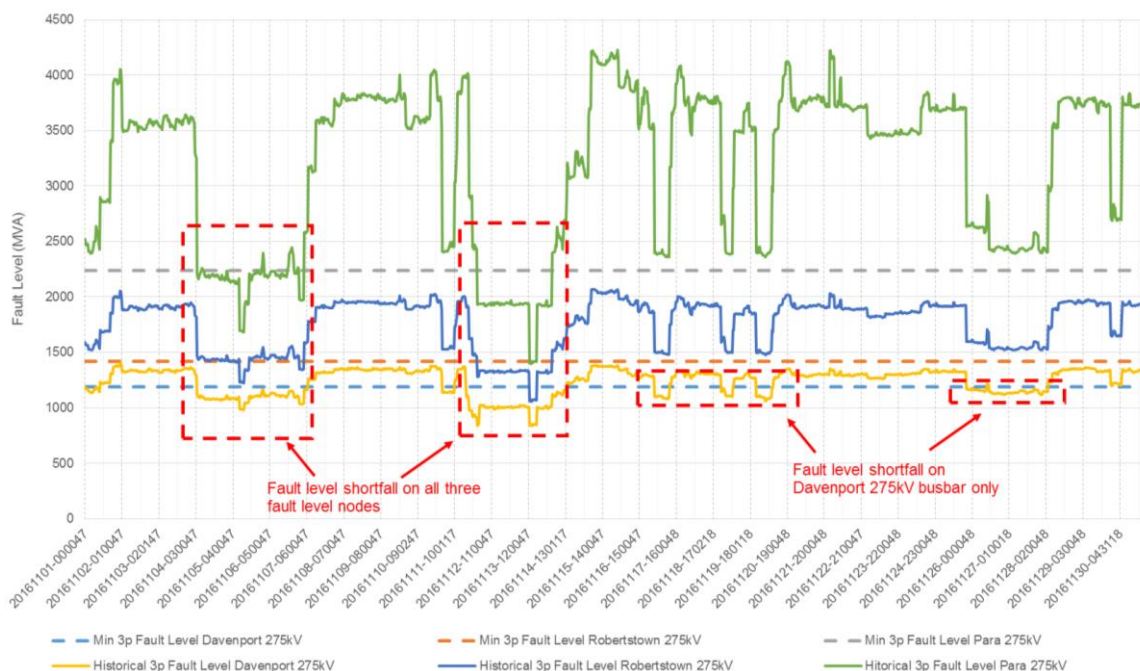
Figure 3 Historical fault level shortfall in SA without AEMO Direction (November 2016)
