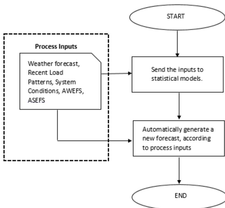
Figure 1 Statistical Model Forecasting Flowchart
