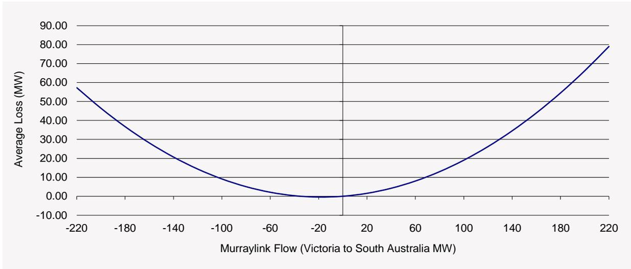
**Murraylink notional link losses versus Murraylink flow (Victoria to South Australia)**
