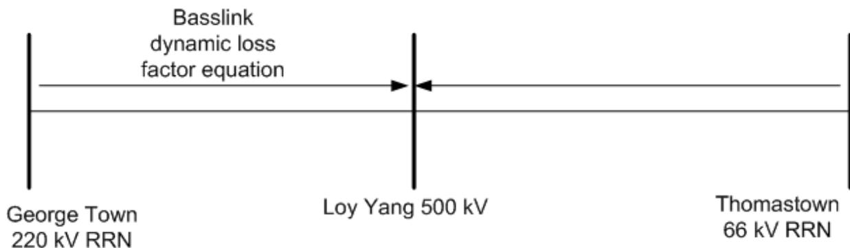
The equation describing the losses between the George Town 220 kV and Loy Yang 500 kV connection points can be determined by integrating the (loss factor equation – 1), giving:
