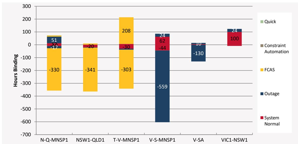
The regional comparison graph below uses the same categories as in Figure 1 as well as non-conformance, network support agreement and ramping. Constraint equations that cross a region boundary are allocated to the sending end region. Global FCAS covers both global and mainland requirements.
