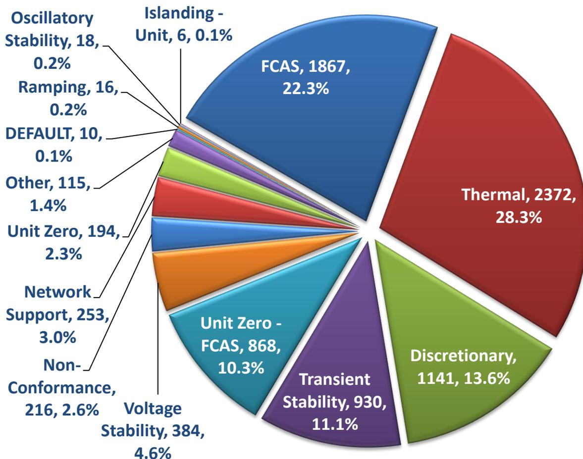
Figure 2: Constraint equations by limit type
