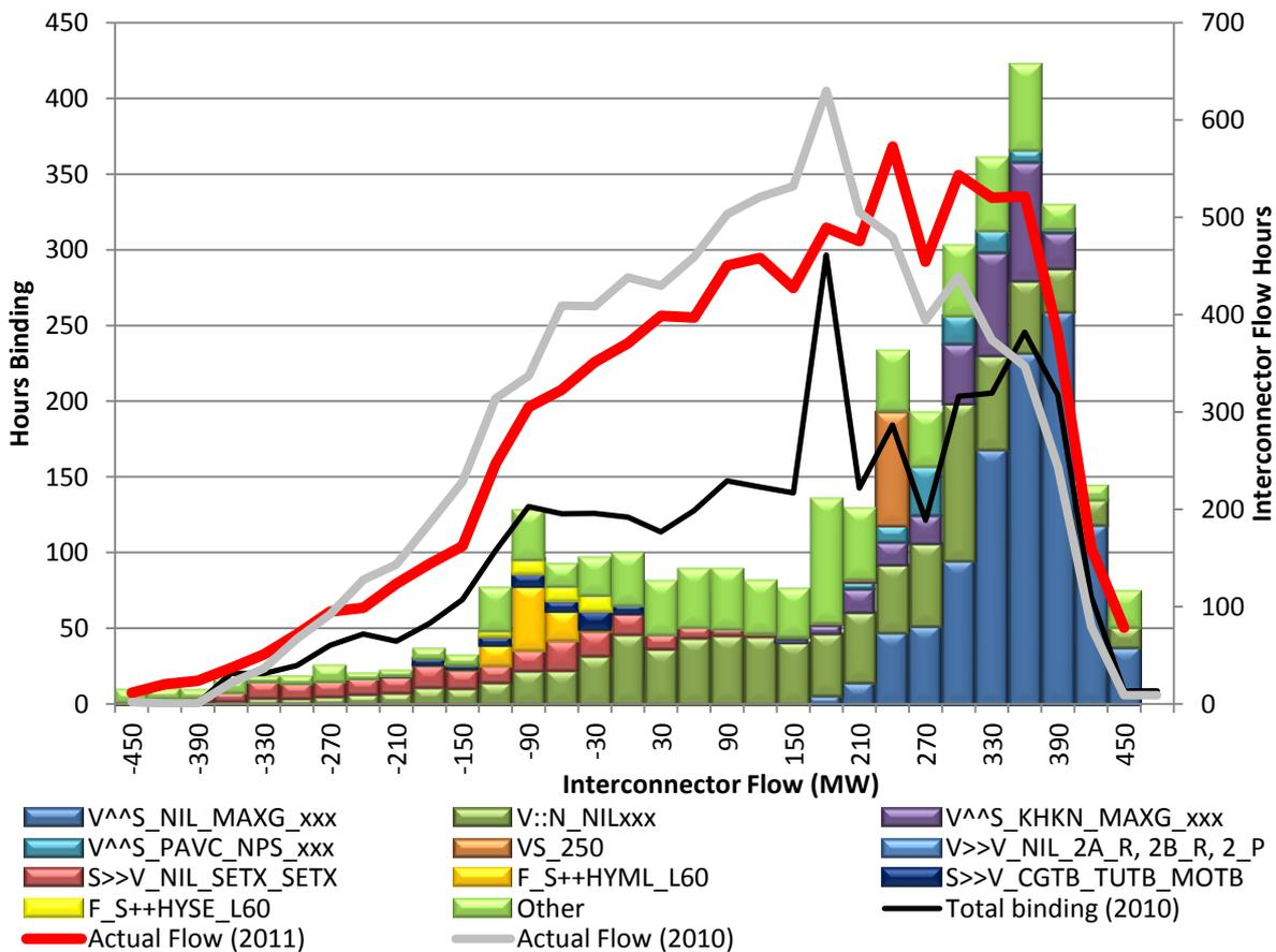
Figure 21: Binding constraint equation distribution for V-SA
