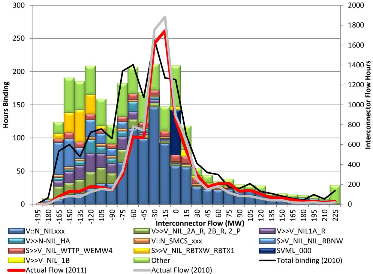
Figure 23: Binding constraint equation distribution for Murraylink
