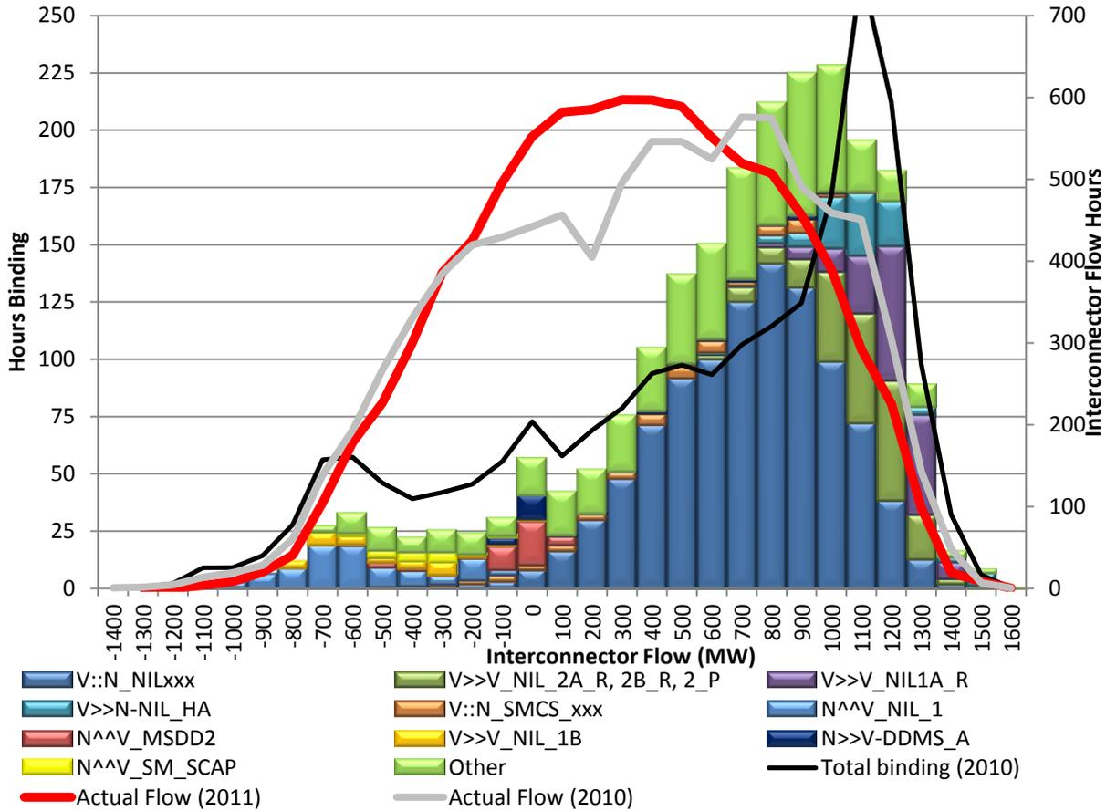
Figure 19: Binding constraint equation distribution for VIC1-NSW1
