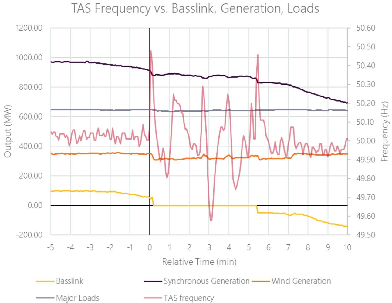
The number of exceedances outside the NOFEB can be further explained by a significant increase of 57% in the energy imported to Tasmania in Q1 2023 compared to Q4 2022 as shown in Figure 9. Additionally, the total import exceeded 400 MW noticeably more in Q1 2023, which suggests that the functionality of Basslink’s frequency controller would have been limited more often in Q1 2023 than Q4 2022.
