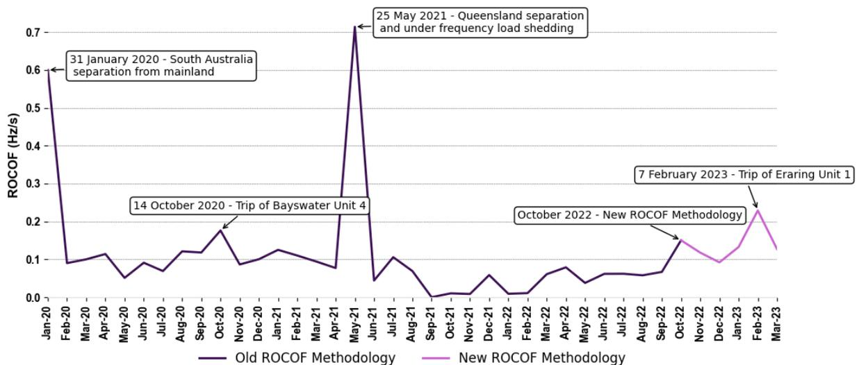
Note: 31 January 2020 RoCoF as measured in South Australia and 25 May 2021 RoCoF as measured in Queensland. New ROCOF calculation methodology used as of October 2022.
