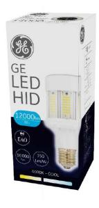
The 80W LED HID lamp from GE offers a safe, cost effective and energy efficient alternative to HID Mercury lamps for outdoor and industrial applications. Direct replacement solution for up to 150W HPS, 100W and 150W CMH, 175W and 250W QMH and 250W and 400W MV lamps.
