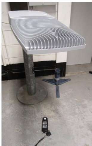
Photo 3. Luminaire during test.
