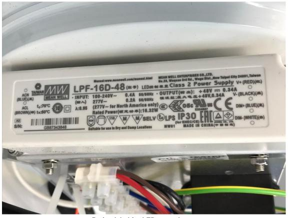
Rating label for LED control gear
