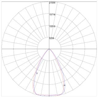
Maximum Candela = 21035.17 Located At Horizontal Angle = 0, Vertical Angle =-13 H - Horizontal Axial Candela V - Vertical Axial Candela
