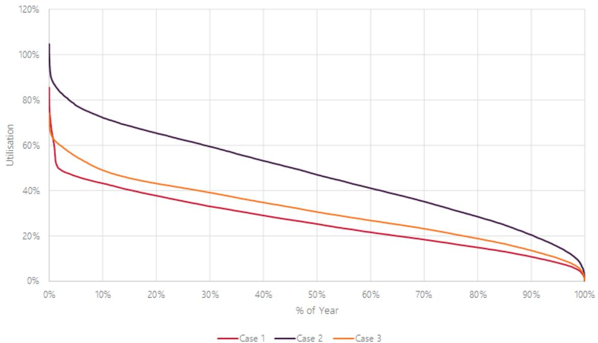
Similar to the RWTS-TTS 220 kV line, the loading on the TSTS-TTS 220 kV line is projected to exceed its rating in radial mode (Case 2) while in parallel mode (Case 3) the loading on the lines is projected to remain within its rating.
