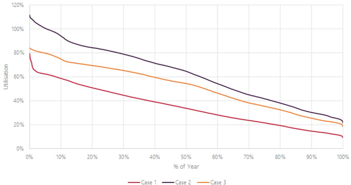
Figure 35 shows that for the cases considered, the loading on the HWTS transformers, under system normal conditions, is below 100% irrespective of the mode of operation. It also shows that utilisation of the transformers is much higher in the cases where the 500 kV and 220 kV networks are operated in parallel (Case 3) than the cases where they are operated radially (Case 1 and Case 2).
