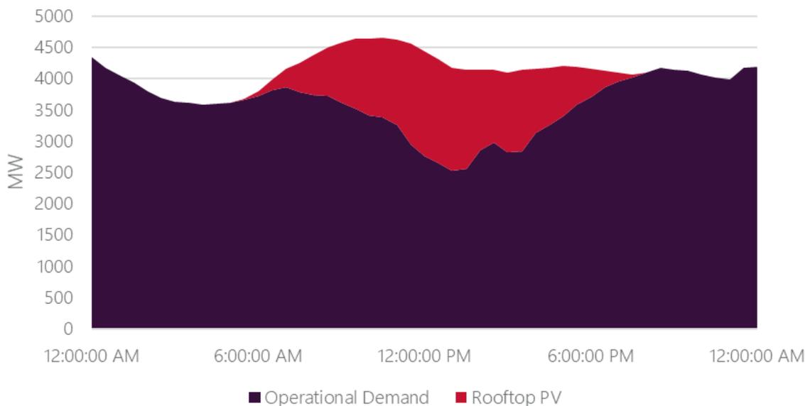
As the capacity of rooftop PV systems increases, minimum demand that has traditionally occurred during the night-time instead occurs during daylight hours while PV generation offsets consumption.
