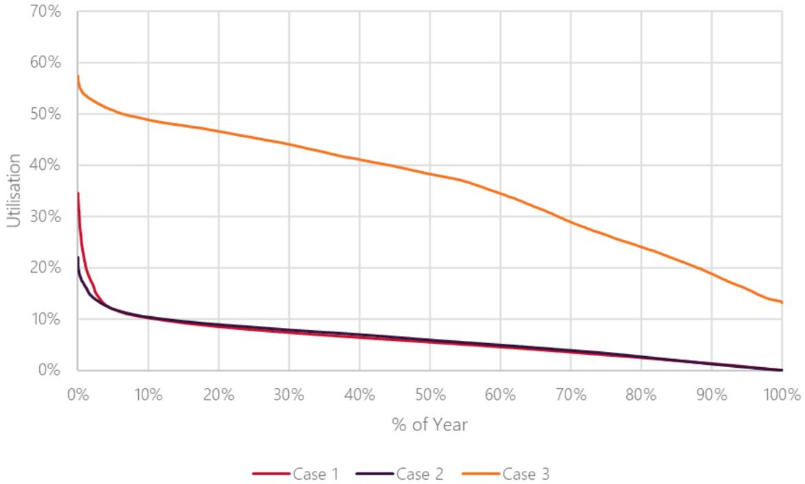
Figure 36 shows that the loading under a contingency, of the HWTS transformers is significantly higher when the network is operated in parallel.
