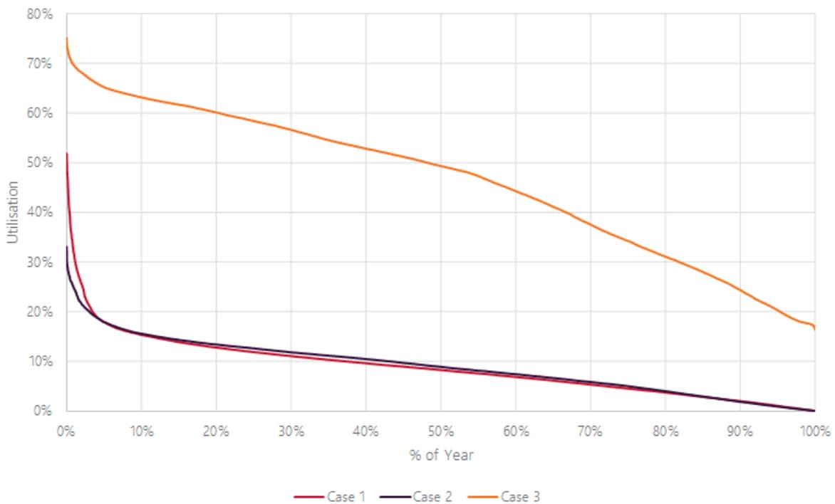
Figure 37 shows that with the 500 kV and 220 kV networks operated in parallel, the loading on the HWPS-YPS 220 kV lines, under contingency conditions, is projected to exceed 100% of their ratings for up to 20% of the time for Case 3. In the radial cases, the HWPS-YPS 220 kV lines are effectively forming a bus tie between the
