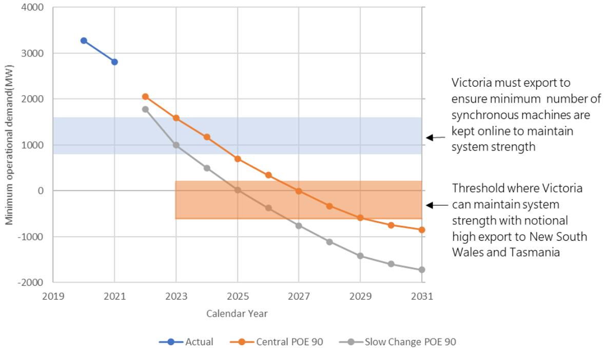
The assumed export capability is 478MW to Tasmania and 900MW to New South Wales based on the published interconnector capabilities.<sup>92</sup>
