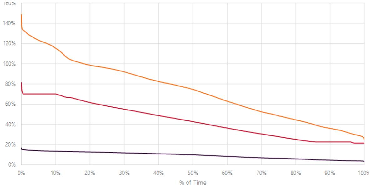
Figure 38 shows with the 500 kV and 220 kV operated radially, the loading on the RWTS-TTS 220 kV line, under contingency, is projected to exceed its rating for a small period of time (Case 2). In parallel mode (Case 3), the loading on the line is projected to remain within its rating.
