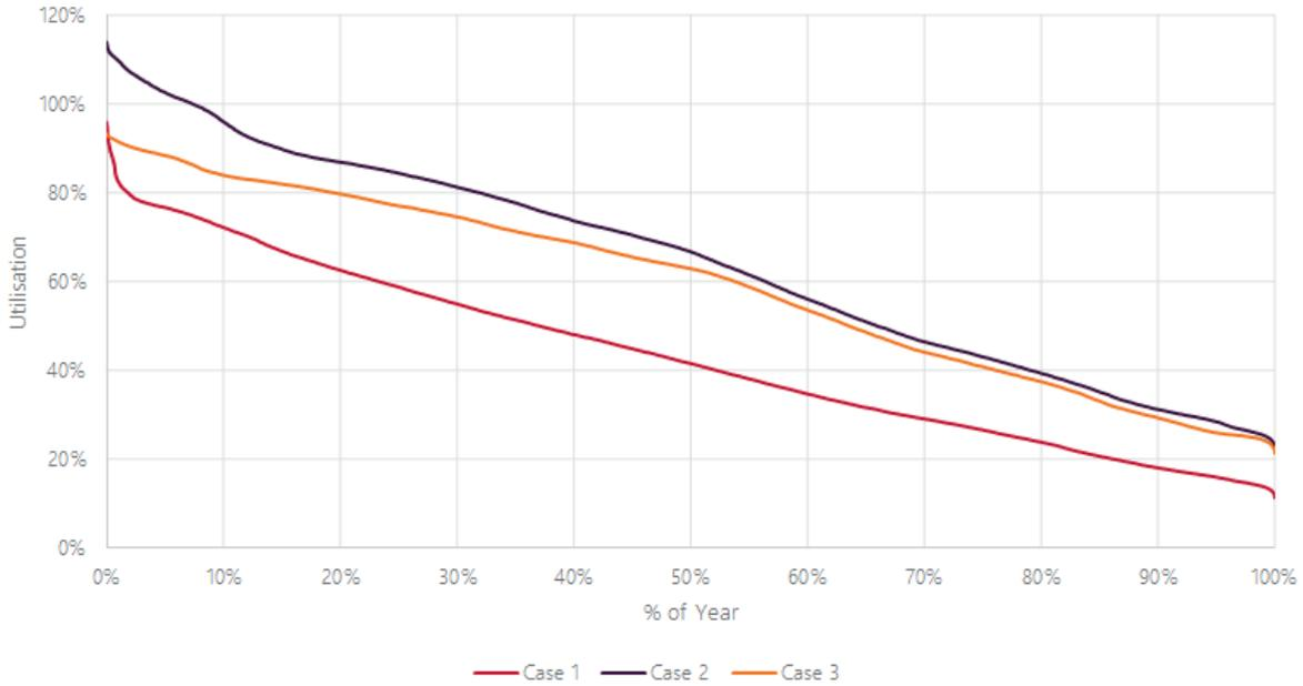
Figure 34 shows that under Case 2, the ROTS A1 transformer is projected to overload approximately 7% of the year. In parallel configuration, the ROTS A1 transformer loading remains below 100% (Case 3).
