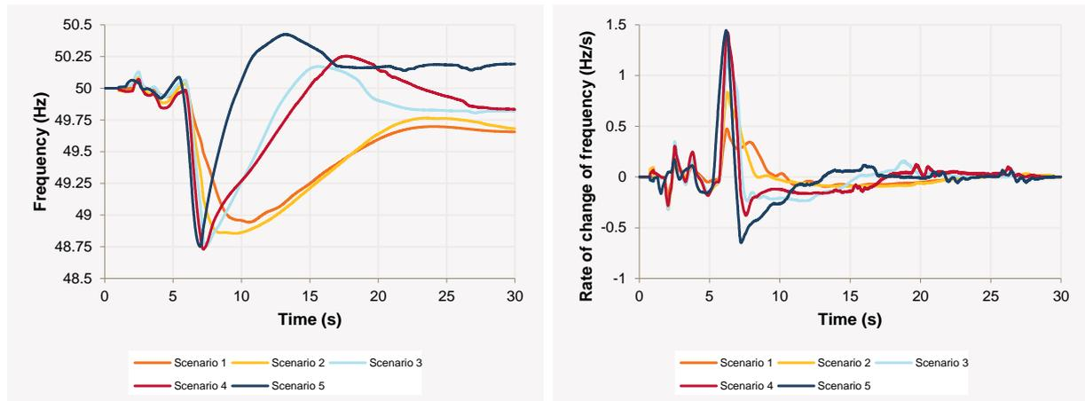
\* Scenarios 1 to 5 reflect varying levels of online synchronous generating units contributing to frequency recovery.
