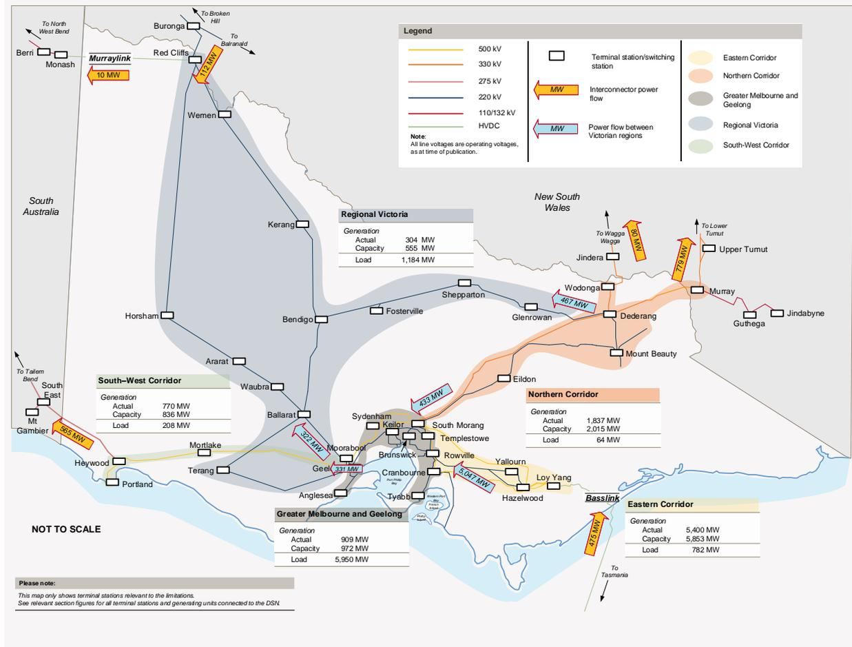
Figure 1 reflects the prevailing conditions at the time of Victorian maximum demand (13:30:47 on 9 February 2017). It shows the electrical regions and their interconnectors, and the transmission lines and their voltages. The arrows indicate power flow from one Victorian electricity region to another, and the lines represent single or multiple transmission lines.
