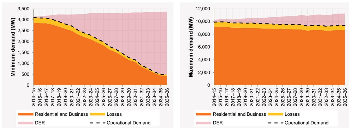
The uptake of DER will provide an opportunity to manage the power system in new ways, particularly when combined with advanced metering and control. If DER uptake is not holistically managed, however, it is likely to have a substantial and unpredictable impact on the power system.
