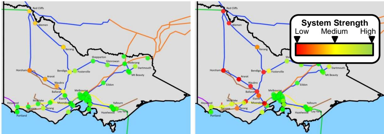
The effects of low system strength on system disturbances are deeper voltage dips, slower voltage recovery, and reduced power quality. The geographic spread and the depth of voltage dips increase as system strength decreases.
