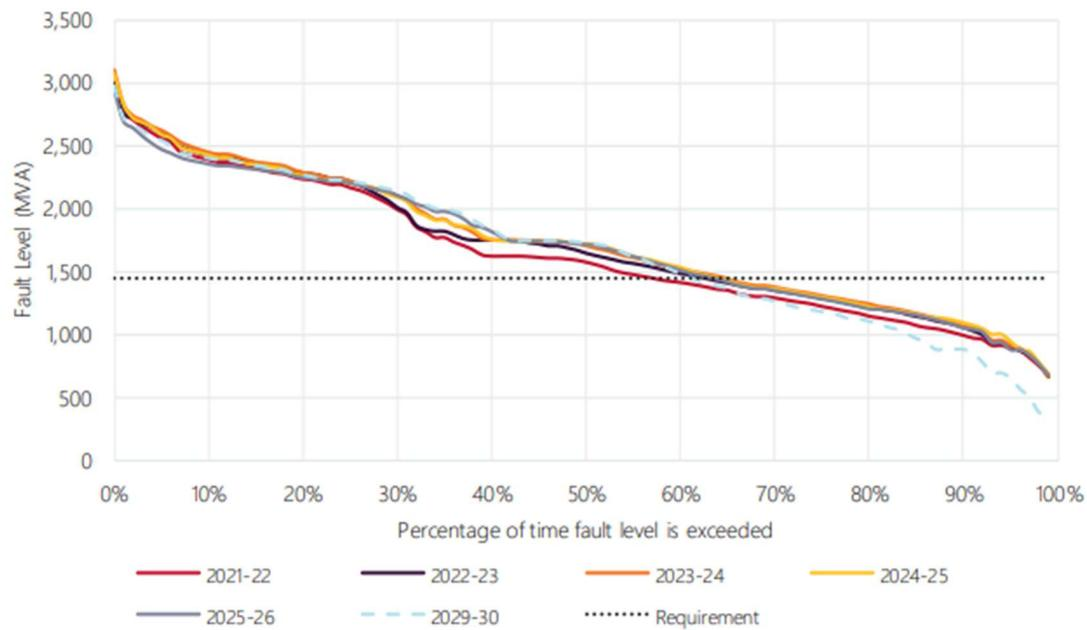
Figure 3 shows the Risdon outlook including fault level below the requirement for 29% of the year in 2025-26, and a worst-case shortfall of 580 MVA (for 1% of the time) across the 5-year horizon.
