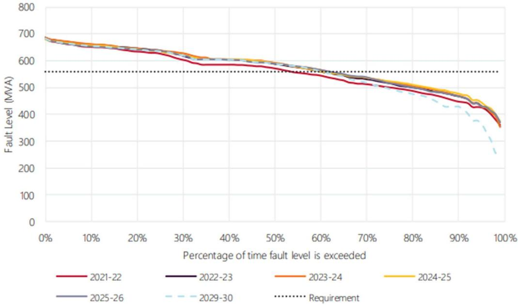
Figure 2 shows the George Town outlook including fault level below the requirement for 37% of the year in 2025-26, and a worst-case shortfall of 770 MVA (for 1% of the time) across the 5-year horizon.
