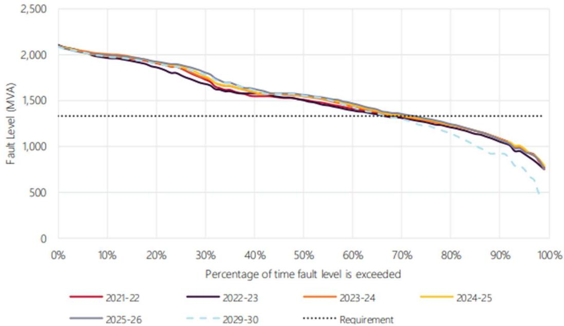
Figure 4 shows the Waddamana outlook including fault level below the requirement for 17% of the year in 2025-26, and a worst-case shortfall of 620 MVA (for 1% of the time) across the 5-year horizon.
