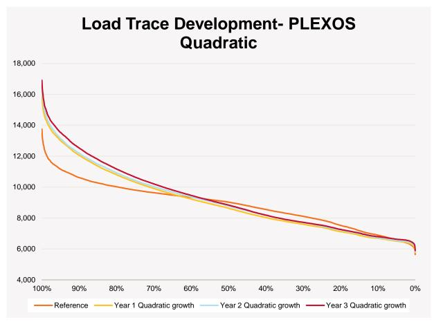
By also including a distortion factor, additional energy could be moved from the mid-high demands, into the mid-low demand range. The final result is shown in Figure 4 below.
