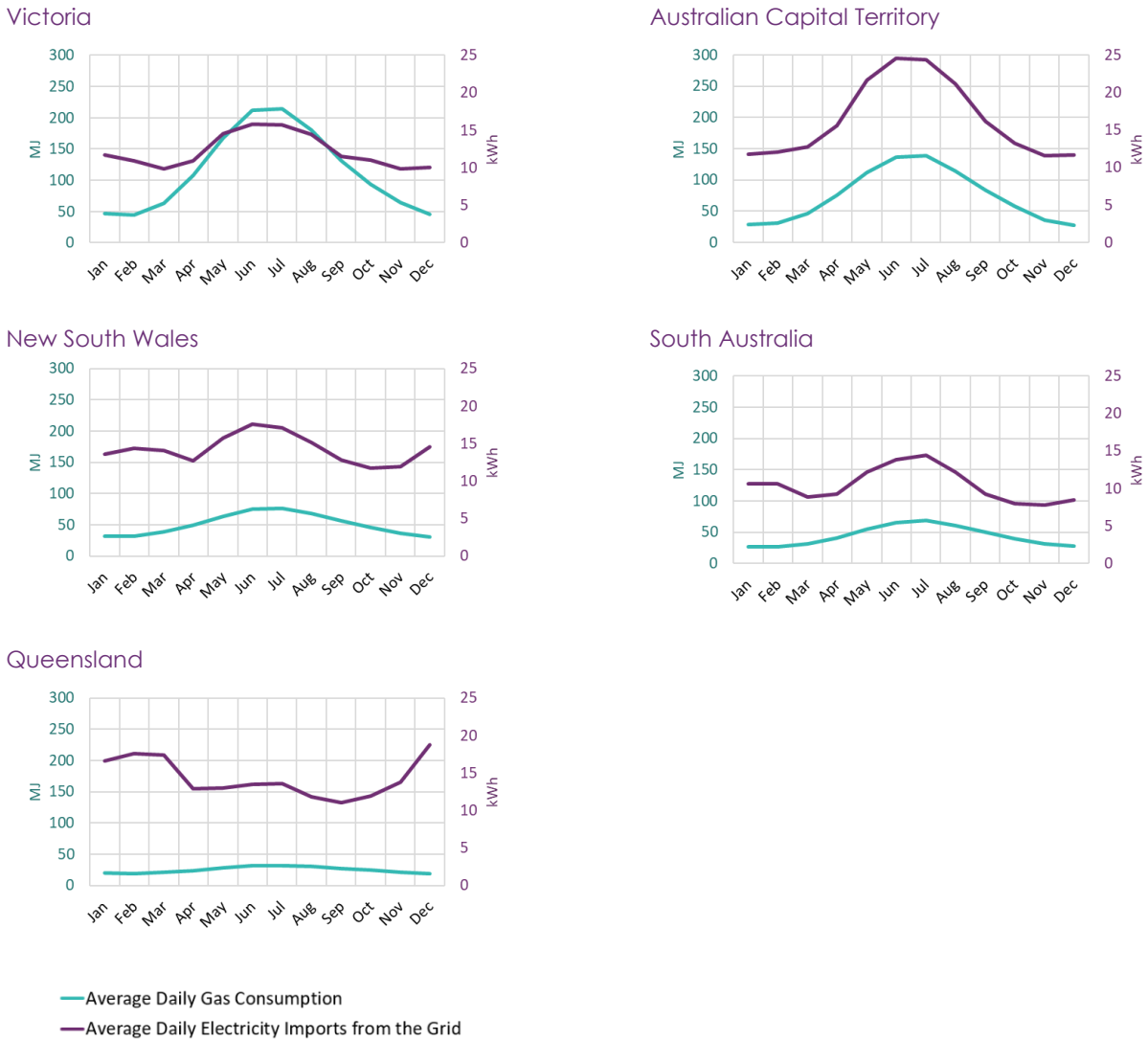
Figure 2 Average daily gas usage and electricity imports for dwellings with a gas connection, by region – 2023 CY
