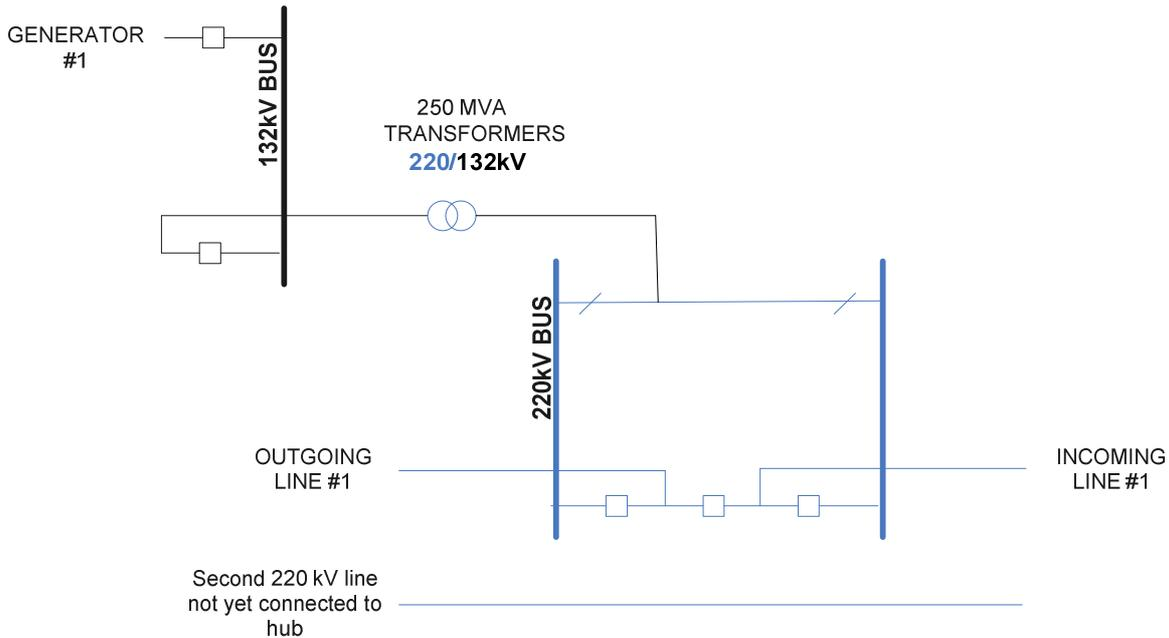
Figure 8: Stage 1 of 220/132 kV Hub to Connect Generation Capacity in the Range 0 MVA - 250 MVA
