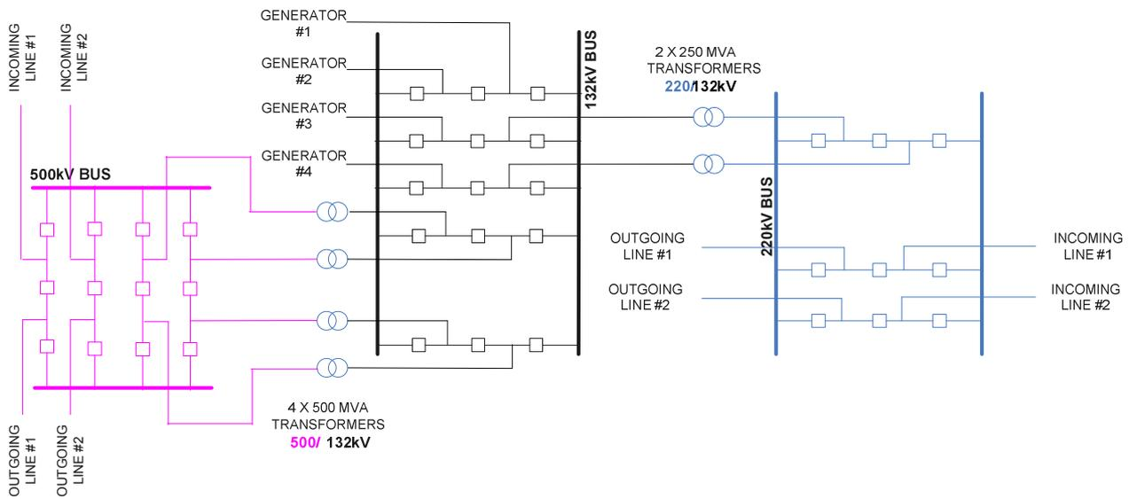
Figure 10: Stage 3 - Ultimate Layout Option for 500/220/132 kV Collector Hub
