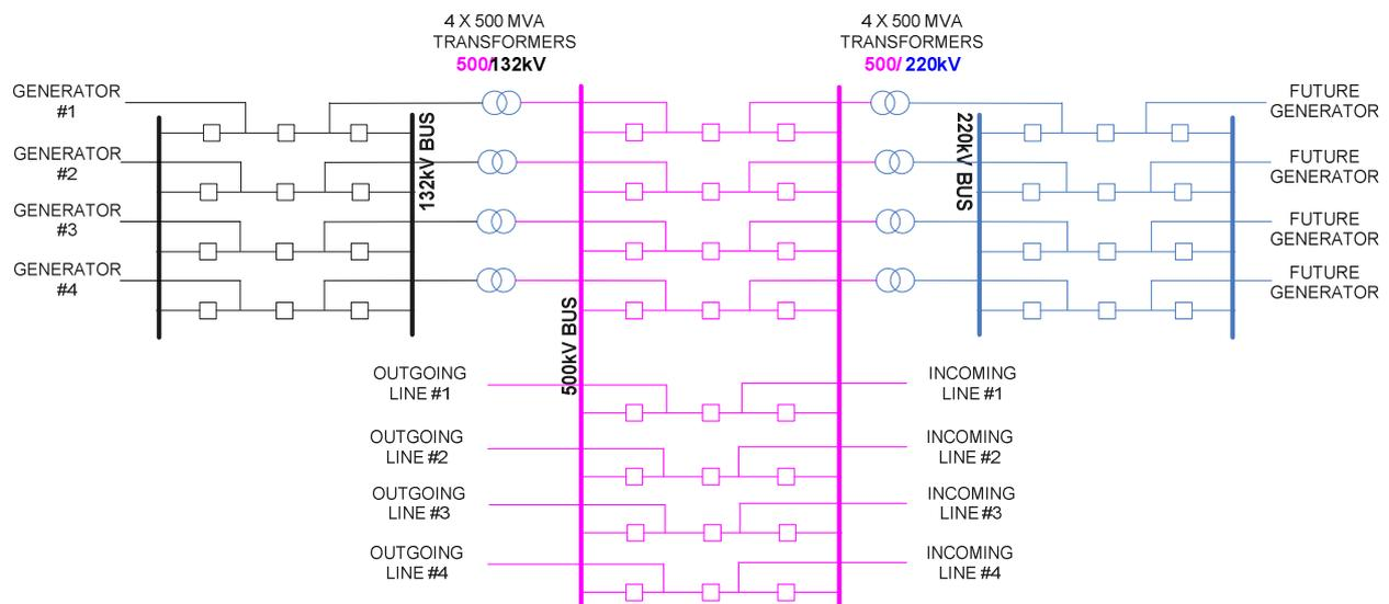
Figure 13: Stage 3 - Ultimate Layout of 500/220/132 kV Hub
