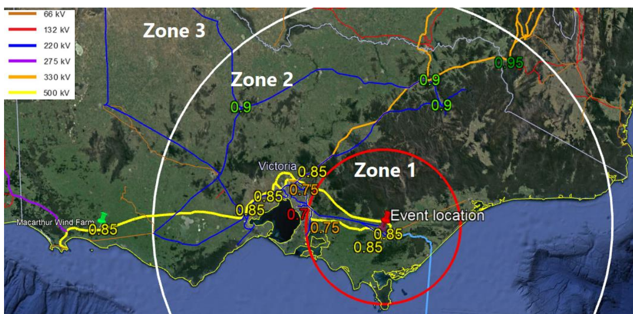
Figure 2 Minimum voltages recorded (pu minimum on a single phase) at the time of fault (13:26 hrs)
