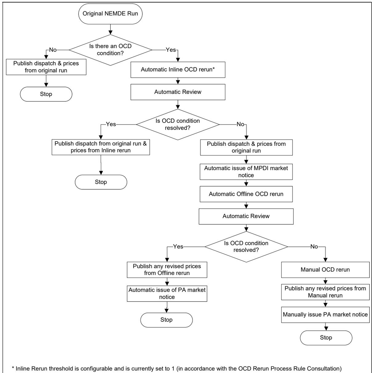
**Figure 1 Over Constrained Dispatch Re-run Flow Diagram**
