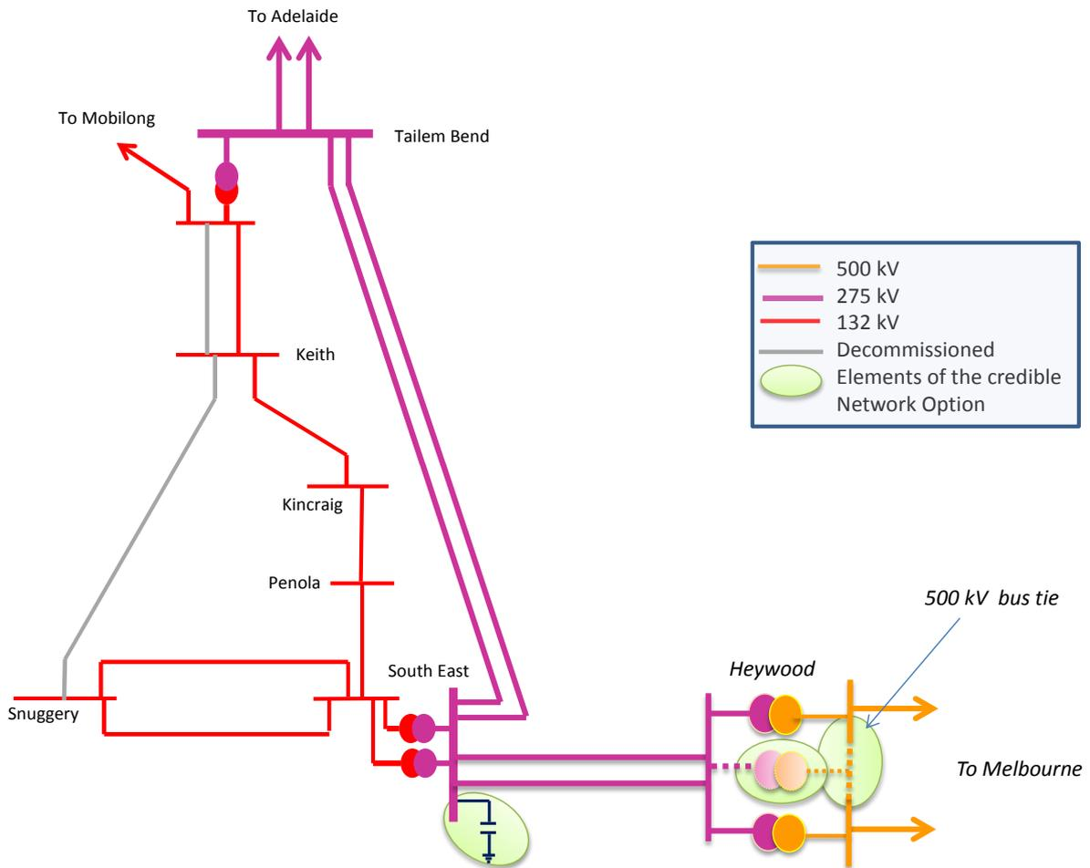
**Option 1b – Installation of a 3<sup>rd</sup> 370 MVA 500/275 kV transformer at Heywood and 500 kV bus tie plus series compensation of 275 kV lines and reconfiguration of 132 kV network**
