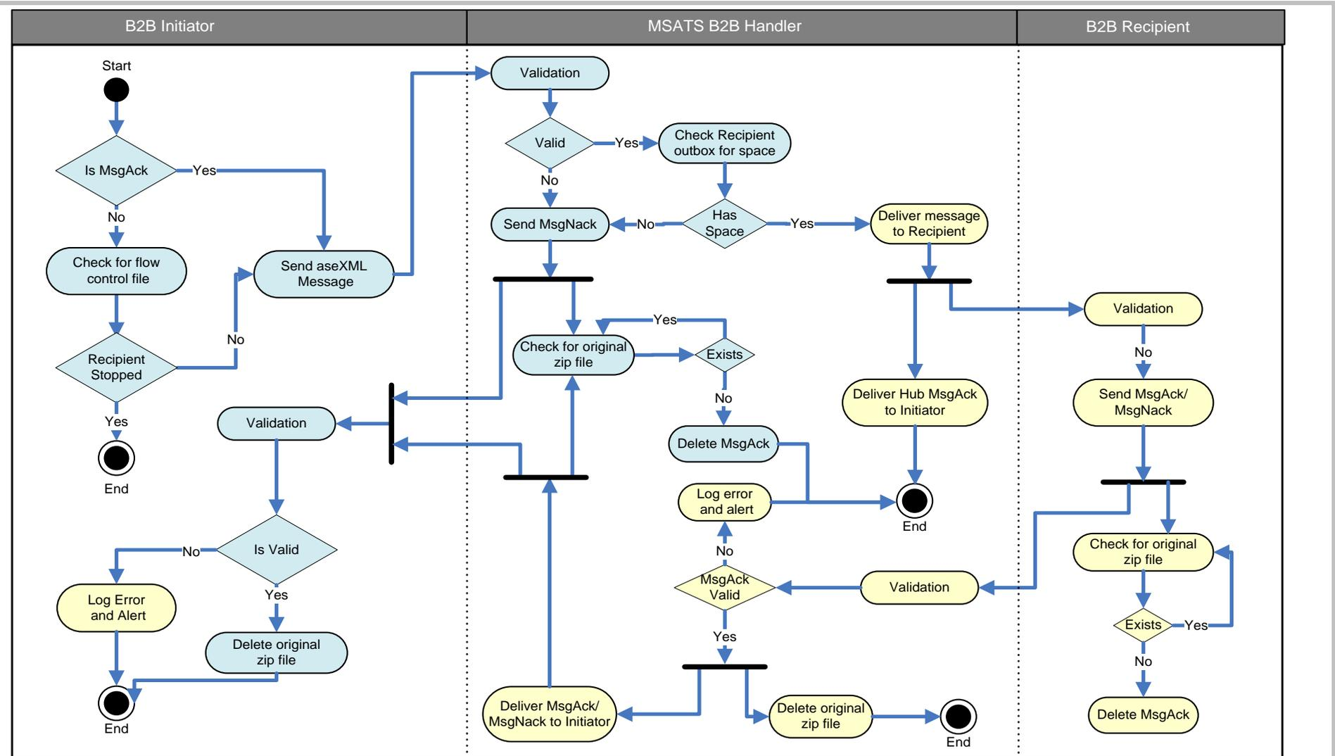
Figure 5: Activity Diagram - Acknowledgement Model for MSATS B2B Handler. Activities and decision points highlighted in blue for scenario where the Recipient Outbox is full when checked by the MSATS B2B Handler.
