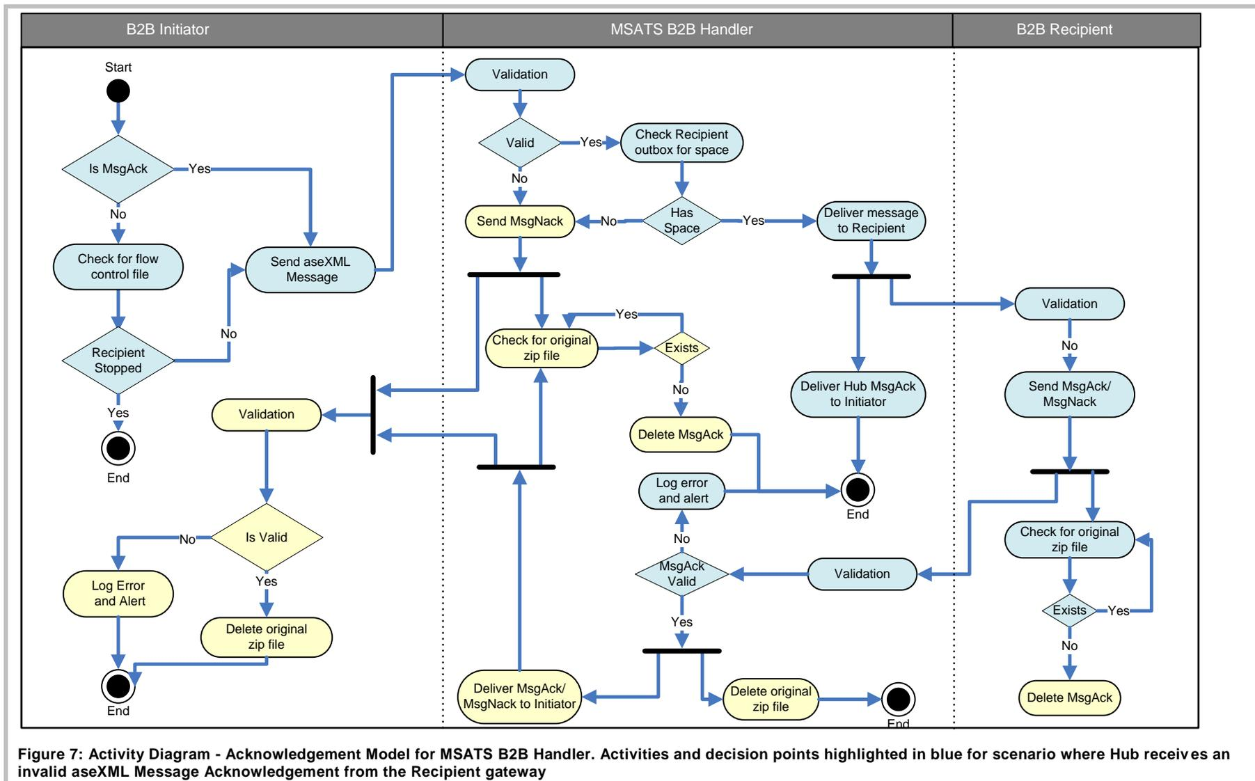
Figure 7: Activity Diagram - Acknowledgement Model for MSATS B2B Handler. Activities and decision points highlighted in blue for scenario where Hub receives an invalid aseXML Message Acknowledgement from the Recipient gateway
