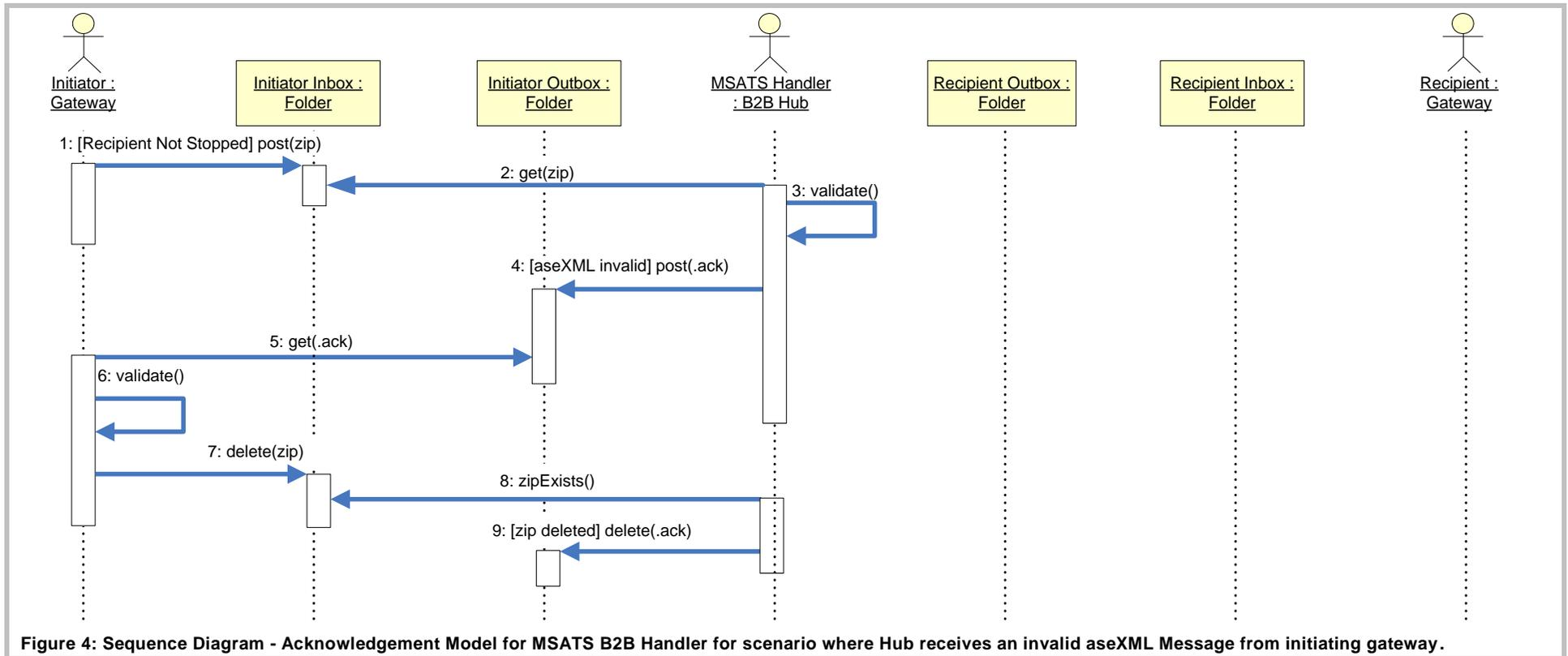
Figure 4: Sequence Diagram - Acknowledgement Model for MSATS B2B Handler for scenario where Hub receives an invalid aseXML Message from initiating gateway.
