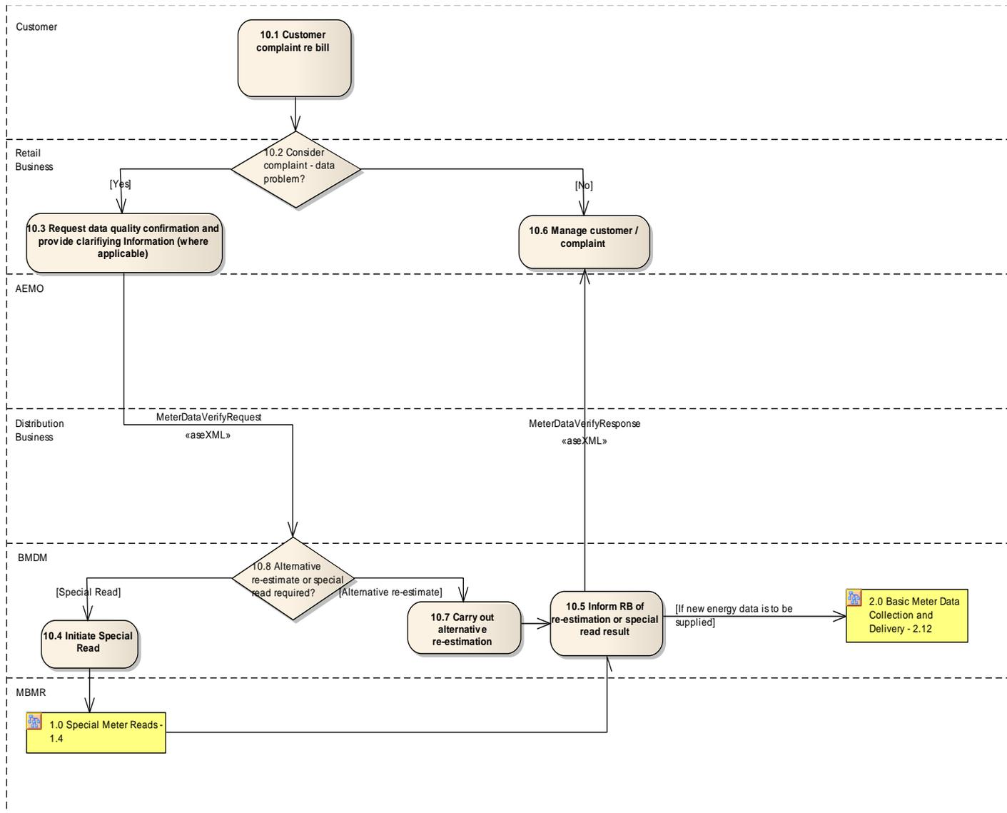
**4.241.16** **DIAGRAM 11.0 – BASIC METER PROFILER (BMP)**
