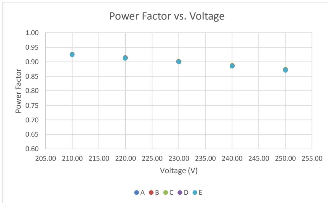
Power factors measured have a Leading phase angle and therefore the driver has capacitive properties.
