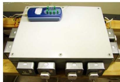
The products under test are connected to the UMS Test system which has full data control and recording using Labview software. This allows full integration of the Test equipment used - Kikusui AC Stable Power Supply , Yokogawa Power Analyser, Pico Temperature Logger and a LUX-TSI distribution control panel
