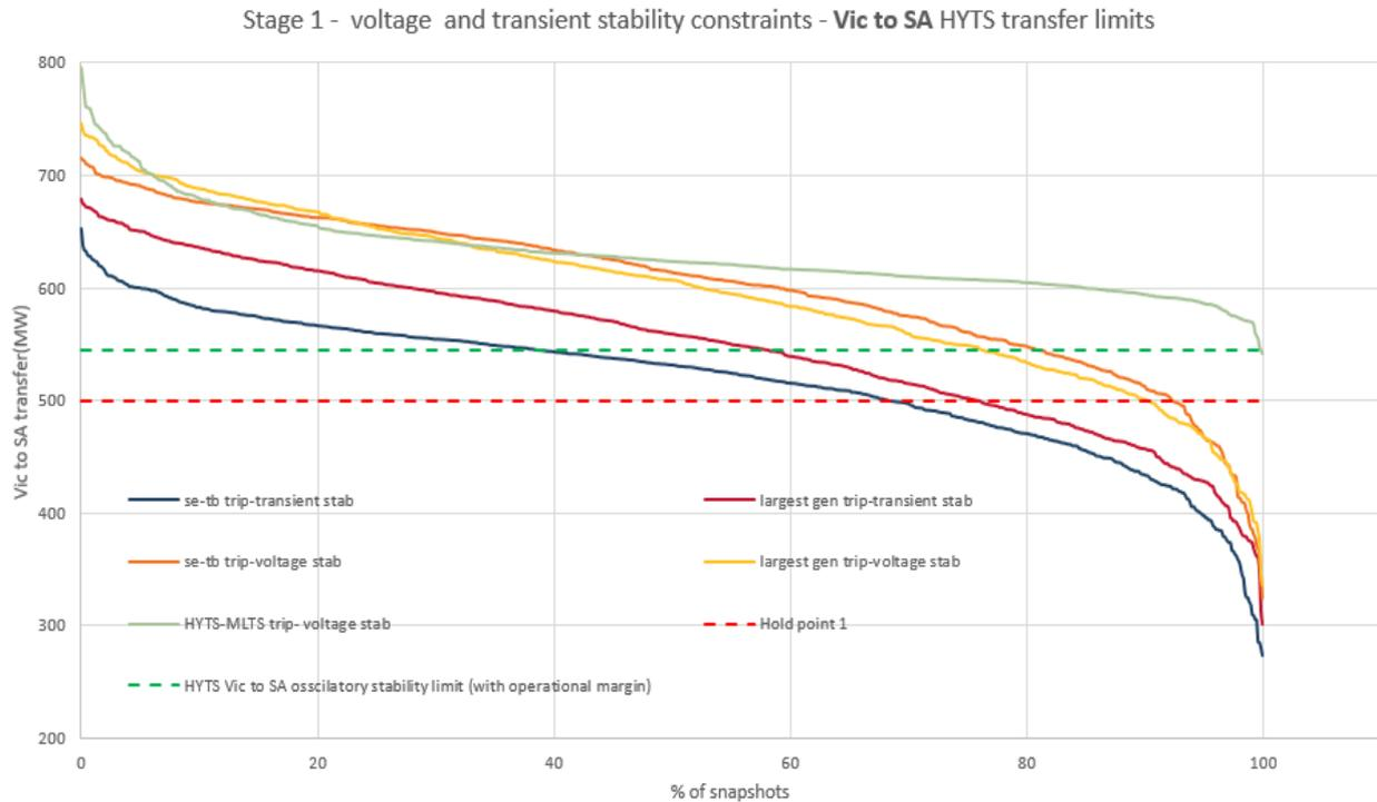
The system normal Vic to SA transient limit via HYTS for trip of a SESS-TBTS 275 kV line is the most restrictive limit over other voltage and transient limits (Figure 4). During the first stage 1 hold point test, the Vic to SA transfer limit via HYTS may be above 500 MW 70% of the time. During the final stage 1 test hold point, the transient stability limit via HYTS for trip of SESS-TBTS 275 kV line may be below the 545 MW oscillatory stability limit 60% of the time.
