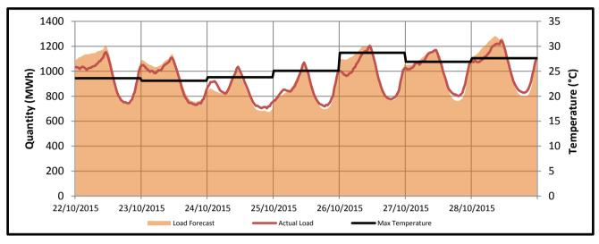
The maximum temperatures for this trading week ranged from  $23.1^{\circ}$ C to  $28.7^{\circ}$ C. The actual load peaked at 1245.129 MWh on the 28/10/2015.
