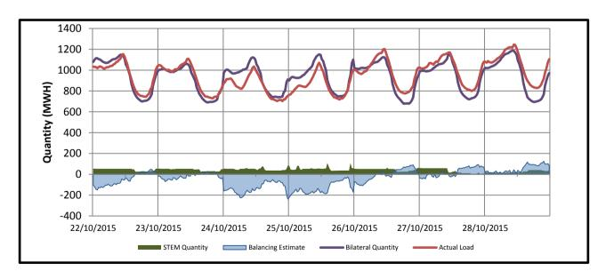
Total balancing supply equalled -18289.075 MWh whereas total balancing demand equalled 5595.863 MWh. The Total STEM Traded quantity was 14022.141 MWh, with the STEM Clearing Quantity ranging between 0.108 MWh and 109.274 MWh.
