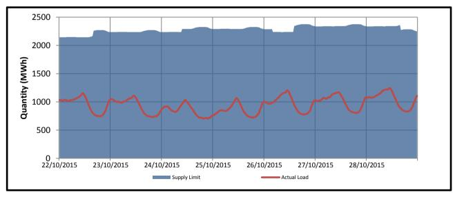
The supply limit ranged from 2144.55 MWh to 2375.821 MWh
