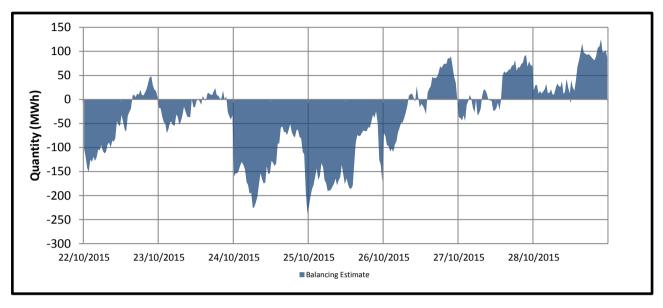
The majority of the balancing activity this week occurred within Balancing Supply. The maximum balancing demand for the week reached 125.2775 MWh on the 28/10/2015. The maximum balancing supply for the week reached -237.657 MWh on the 24/10/2012.
