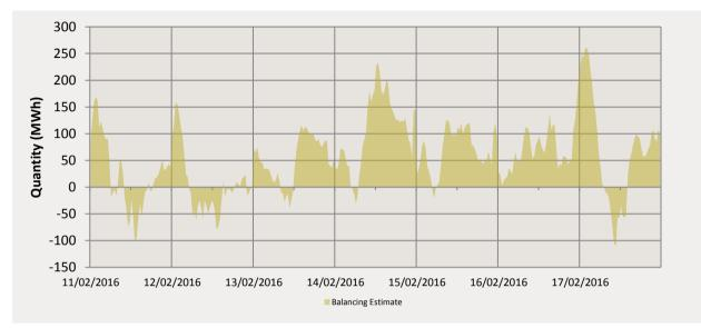
The majority of the balancing activity this week occurred within Balancing Demand. The maximum balancing demand for the week reached 261.458 MWh on the 17/2/2016. The maximum balancing supply for the week reached -110.101 MWh on the 17/2/2012.
