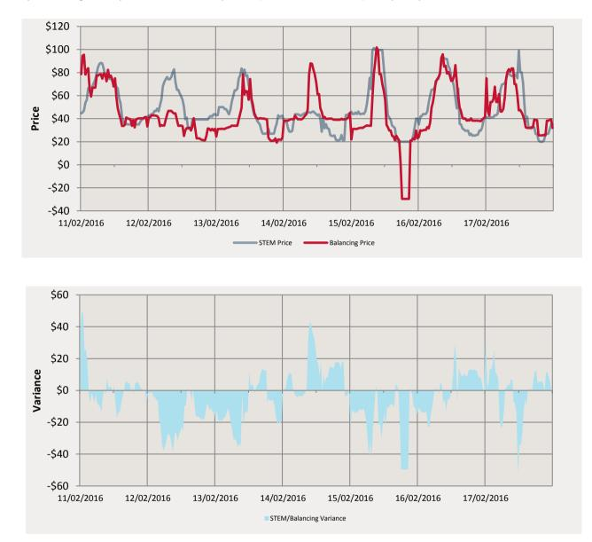
The maximum STEM price was \$101.23/MWh on the 15/2/2016 and the minimum STEM Price recorded was \$20/MWh on the 17/2/2016. The maximum Balancing price was \$101.81/MWh on the 15/2/2016 and the minimum Balancing price recorded was \$-29.61/MWh which occurred on the 15/2/2016.
