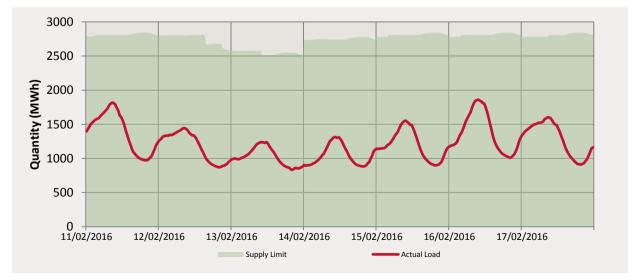
The supply limit ranged from 2514.728 MWh to 2840.42 MWh
