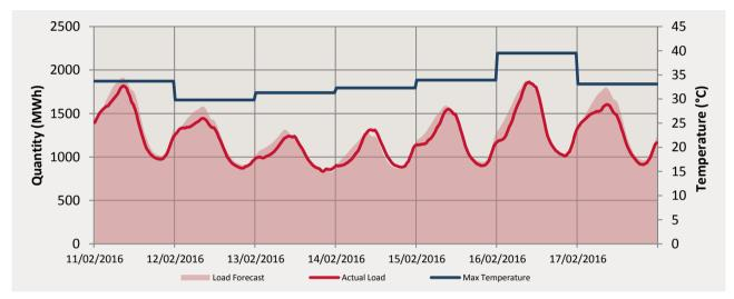
The maximum temperatures for this trading week ranged from 29.8°C to 39.5°C. The actual load peaked at 1862.884 MWh on the 16/2/2016.
